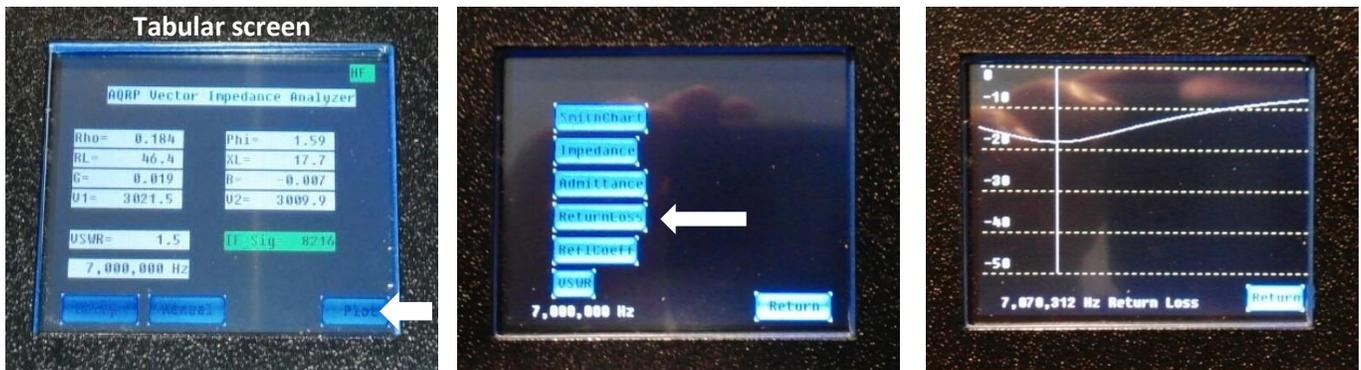
In this test there is only one scale, and rotating the “**Cursor Control**” to the lowest location on the graph will identify the frequency of the lowest reading on the plot. Again this should be close to the lowest VSWR measurement frequency. See the definition for **Return Loss** for more details on this graph.
