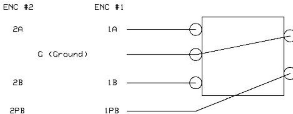
If the Encoder works in reverse, just flip the A and B leads
