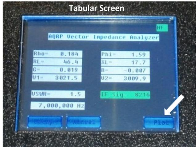
Please note, there should be numbers showing up in all the fields in the "Tabular" screen, and especially in "V1", "V2", and "IF\_Sig" fields. Oh and yes, there must be a load connected to the VIA for it to read correctly. Please connect the antenna to the VIA. ☺ If the fields do not show any varying numbers, please refer to the "Tabular Screen Issues" in the Trouble Shooting section for more help.
