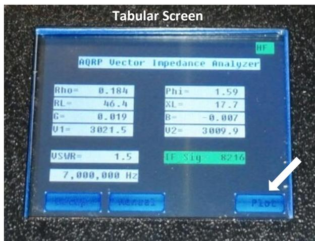
Please note, there should be numbers showing up in all the fields in the "Tabular" screen, and especially in "V1", "V2", and "IF\_Sig" fields. Oh and yes, there must be a load connected to the VIA for it to read correctly. Please connect the antenna to the VIA. ☺ If the fields do not show any varying numbers, please refer to the "Tabular Screen Issues" in the Trouble Shooting section for more help.
