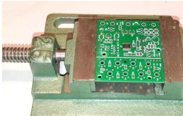
5 – Use a Vise, Helping Hands or some device to hold the **PCB** flat when installing the parts.
