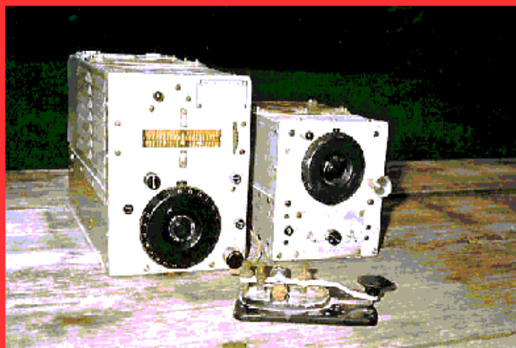
FIGURE 2 – 40 Meters Station Used By K4VOW In 1960 able to KN4VOW. Power supply limitations produced only 25 watts input to the transmitter with approximately 15 watts output.
