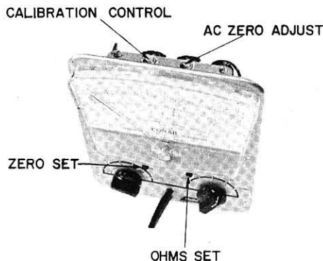
FIG. 1. Model 211 VTVM showing the calibration controls.
