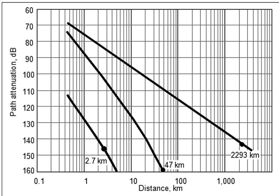
Figure 2—Propagation laws for a 5 W VHF handheld transceiver: (top) by free-space law to a spacecraft; (middle) by suburban law to a repeater tower; and (bottom) to another handheld transceiver at street. The dots indicate maximum range.
