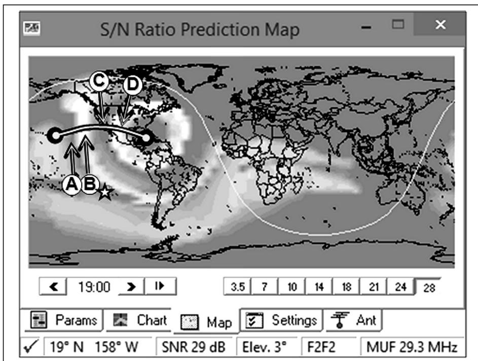
Figure 3—HF propagation prediction at 28 MHz between a transmitter in Florida and receiver in Hawaii. The signal on the ground peaks at D, B, and Hawaii, but skips over C and A. The Sun (star) is roughly midway between the two end points. [Source: HamCAP software by VE3NEA].
