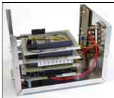
Fig 2—A picture of my “sandwich” construction before I converted several circuits to PLDs.
