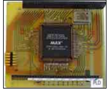
Fig 11—The circuitry of the eight-channel logic analyzer achieved with ICs (left) or a PLD (right).
