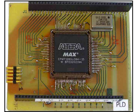
Fig 11—The 8-channel LA board and the PLD board. Notice the two board-stacking connectors on the PLD board.
