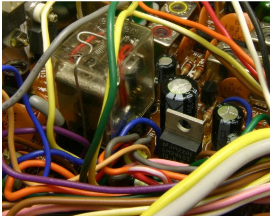
The LM2940-10 used for the regulated RX supply (which is now 10V, not 9)
