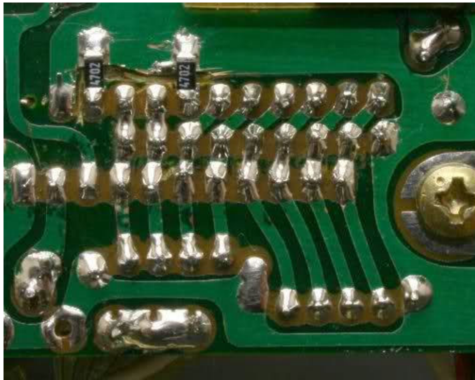
Track cuts were from the 70's, but we replaced the huge old-school resistors with the modern surface mount variety.
