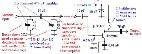
T50-6 powdered iron toroids with 8 turns will tune 15 through 10 meters. T50-2 toroids with 14 turns will tune 40 meters through 15 meters. 160 meters and below requires LARGE inductors. A T-68-15 ( $A_L = 180$ ) with 35 turns will cover 60, 80 and 160 meters. A clever idea is to put 3 toroids in series so that they are equivalent to the lowest frequency toroid. Then for each range, you short the appropriate nodes to ground.
