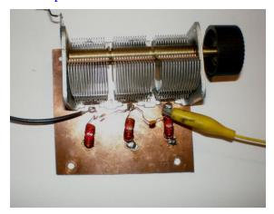
The toroid inductors determine the tuning range. Sadly, it doesn't seem to be possible to cover 160 meters to 10 meters with one set of inductors. If you can figure out the needed complicated switching system, you can cover the entire HF spectrum with 2 ranges of tuning. At this point in my R&D I was soldering in different coils - not very convenient. The inductors described below on the diagram are the most versatile I have tried, they cover 80 meters up to 15 meters.
