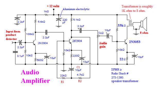
Nearly any crude amplifier will work OK for listening to CW. But if you want to listen to AM and FM voice and music, it is essential that the amplifier be **high fidelity**. In other words, the audio signal delivered to the loudspeaker must be a sequence of smooth, wavy sinewaves. Triangle waves and square waves have sharp angles. They sound terrible and distort speech. Also, in order to listen comfortably with a speaker, it must be **loud**.
