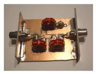
Ideally, filter like this can be switched into the radio whenever needed. The best location is at the antenna signal input to the mixer stage. The desired mixer inputs are the VFO and antenna signals that are *NOT* 6 MHz. The receiver pre-selector is adjusted to capture desired signal frequencies that are either 6 MHz **below** or **above** the VFO frequency.
