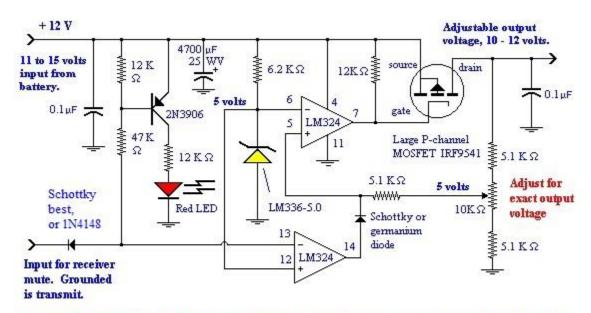
Low Dropout 12 Volt Power Supply with Mute Capability
