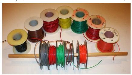
Electrons don't care about the color of a wire's insulation. However, wiring a circuit and trouble-shooting it is *much* easier if we use different colors for different functions of the circuit. Establish your own color codes for positive voltage lines, negative voltage wires, ground wires, active signal wires, etc. For example, I use green or black wires for ground. I connect the positive pole of the power supply with red wire. Define insulation colors any way you like, just be consistent!
