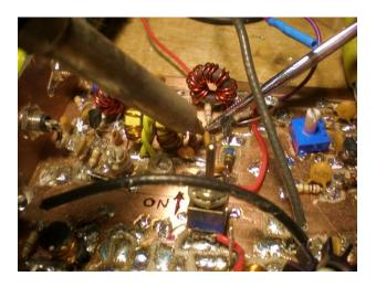
In the photo above, a hemostat coming in from the right is clamped onto 1/4 watt resistor lead. The soldering iron is held in the left hand. As always, holding the solder with your teeth or un-used fingers is a contortion act. At least with the hemostat, you don't have to maintain pressure on needle nose pliers to keep a grip on the wire. Best of all, you won't burn your fingers.
