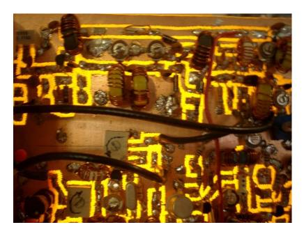
Another advantage of single-sided boards is that the unwanted capacitance between the traces and ground can be very low. This makes single-sided boards practical at VHF frequencies, such as 6 meters (50 MHz) and above.
