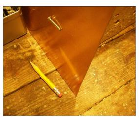
The photo below shows the same steel screw stuck to the magnet directly. Without the 1/16 inch separation caused by the PC board, the attraction is significantly stronger and the screw will stand on end. This obvious attenuation is mostly simply because of the distance. The strength of the magnetic attraction falls off as the inverse square of the distance, 1/(distance)<sup>2</sup>.
