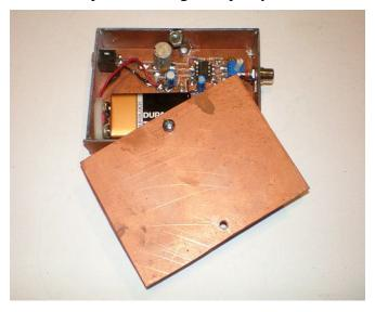
The photo above shows a totally shielded audio amplifier. I built it in a desperate attempt to keep 60 Hz AC hum out of the audio modulation in my 2 meter FM transmitter. It didn't work. It's a nice box, though.
