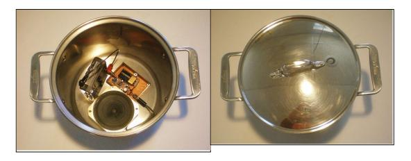
When I placed the apparatus in the stainless steel pot without the lid, the music was still loud and clear but harder to tune in. When I keyed the 147 MHz transmitter, the interference was the same when the transmitter was above the pot, but it was attenuated to a degree when the transmitter was off to the side of the pot. In other words, when there is a metal wall between the antenna and the FM radio, the FM radio signal will be attenuated.
