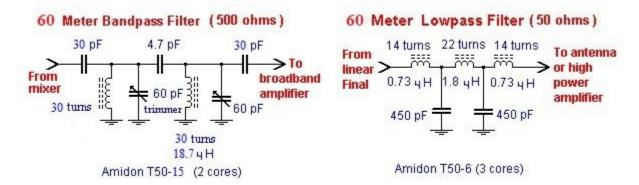
I combined my 40 meter SSB driver with the 60 meter SSB driver. You'll notice that I used the same output low pass filter for both bands. A single DPDT switch allows me to switch between 40 and 60 meters. In all the other double band drivers, two DPDT switches were needed.
