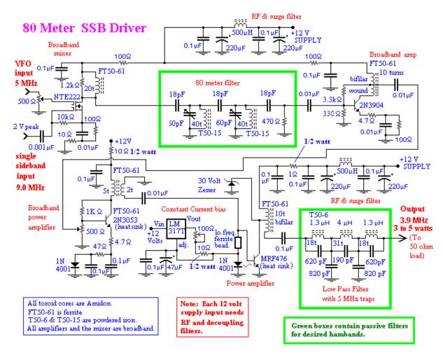
All transistor stages are broadband, including the mixer. Note the 1.2K resistor across the primary of the mixer ferrite core transformer. Without this or other feedback device, the
