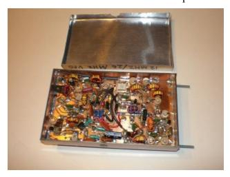
The 12 MHz VFO converter is on the left side of the circuit board. I later added the 26 MHz VFO converter for 17 meters on the right side. The blue DPDT switch to the left of center switches between the two converters. One operational difficulty I had with the 15 meter VFO on the SSB portion of the 15 meter band is that 21 MHz, is the fourth harmonic of the 5.250
