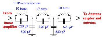
Yes, adding the capacitors achieved the object of getting rid of the 5 MHz signal. Unfortunately, it also degraded the low-pass performance of the filter. Higher harmonic frequencies are now able to motor on right through those three series capacitors. In short, be sure to use a high frequency TVI filter like the one in Chapter 9. Alternatively, you could add another
