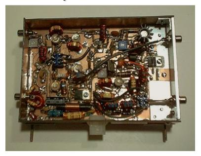
The two large RF choke inductors at the lower left filter the separate 12 volt DC lines for the frequency generator circuits and the final amplifier stages. The large P-channel MOSFET transistor just above the Molex connector and RF chokes turns on the power to the final amplifier keying when the microphone is keyed.
