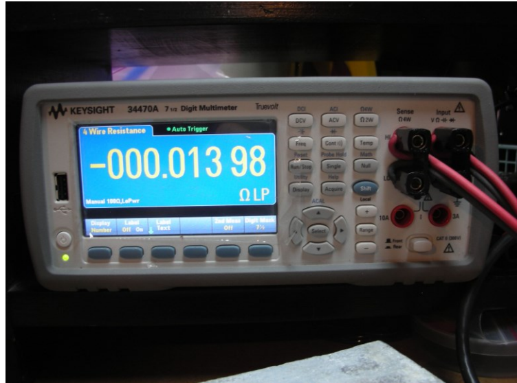
The meter measures the test lead resistance (each wire is 18 awg)
