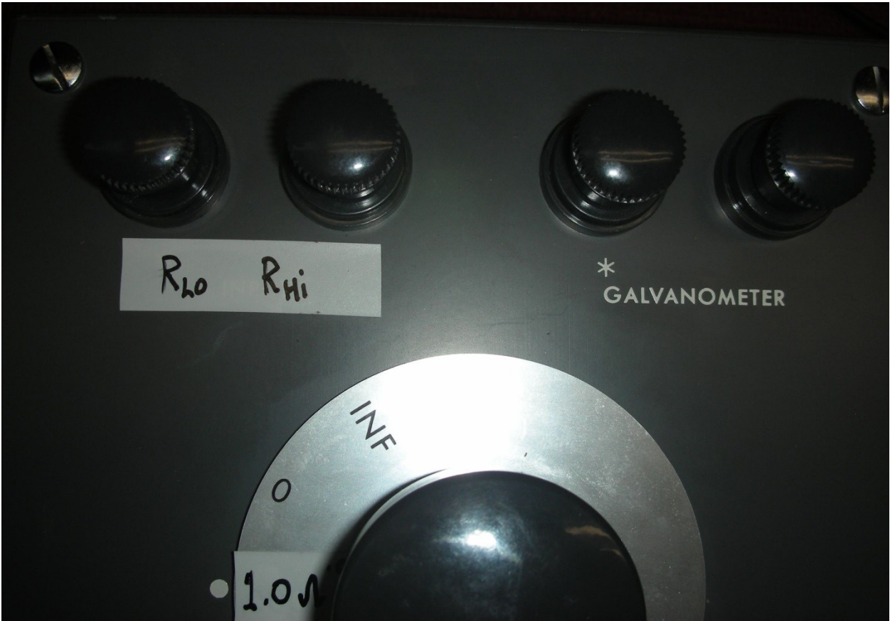
Fig.7- Relabel the original INPUT terminals as R HIGH and R LOW. These is the new Resistance Output terminals.
