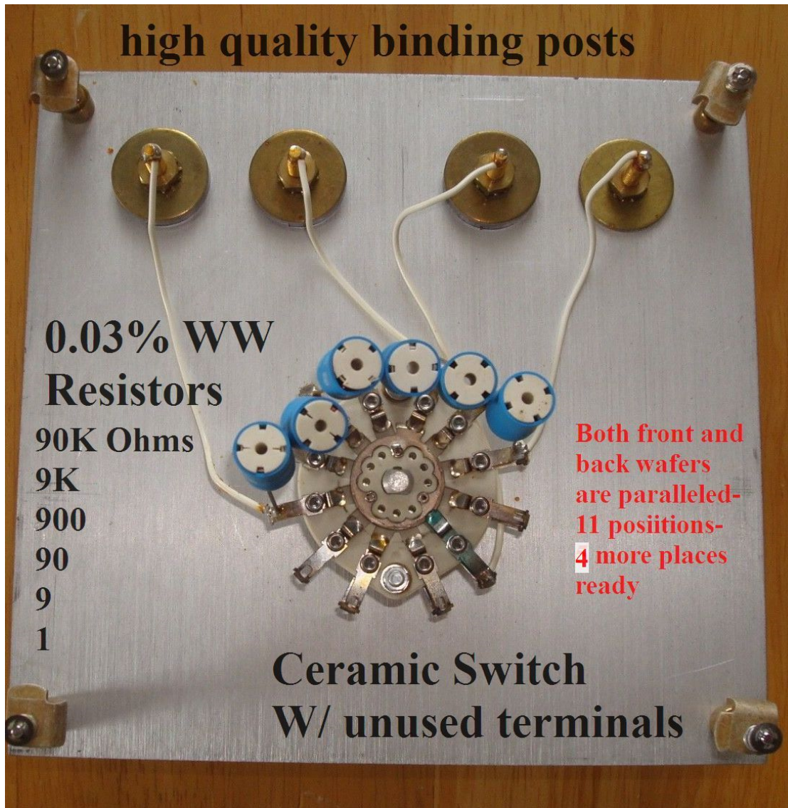
Fig.3- Rear of front panel-switch, Leeds & Northrup 0.03% Wire Wound resistors, wiring and terminals
