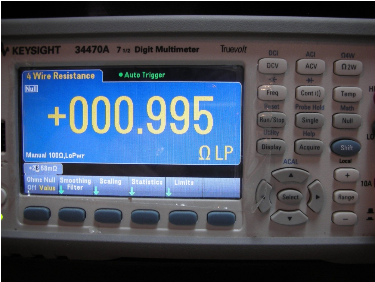
Fig.9- Direct measurement of the 1 Ohm resistor shows it a little low.
