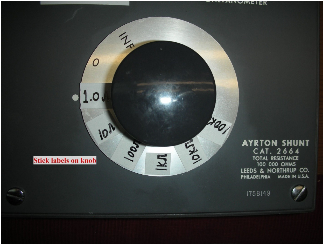
Fig.6- Relabel knob positions to indicate the actual resistance present at the new R OUT terminals.
