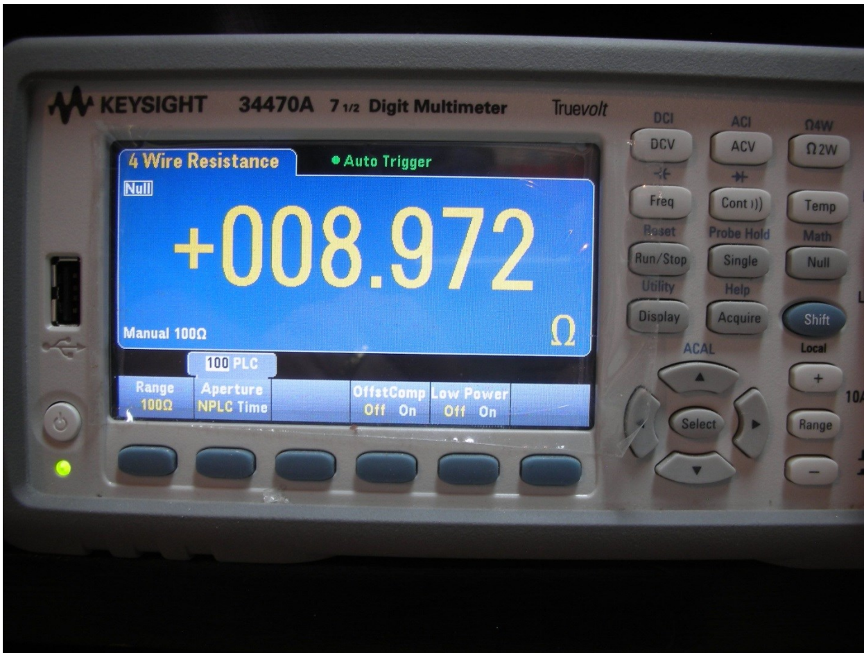
Fig.11- Direct measurement of the 9 Ohm resistor is also slightly low.
