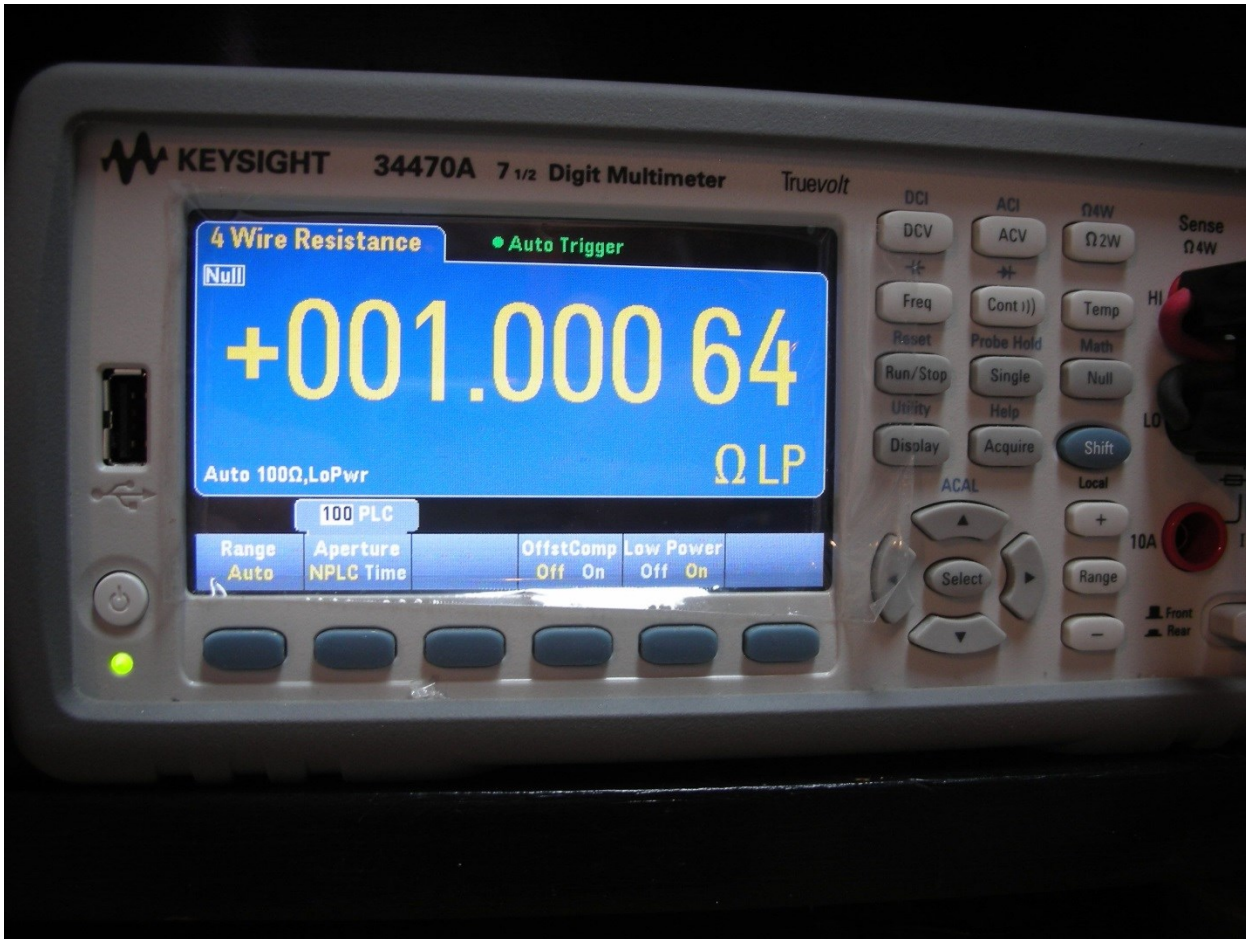
FIG.10- But add in the extra resistance of wiring and switch contacts, at the terminals it is perfect!
