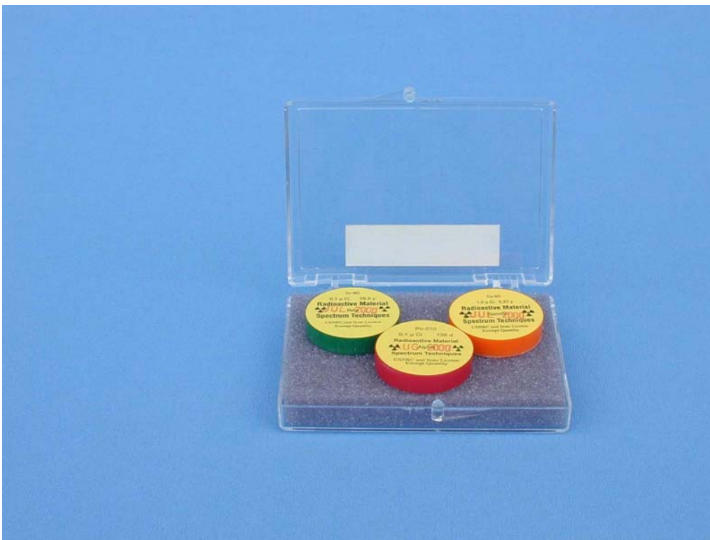
Figure 2 – Kit with one each of an alpha emitter, beta emitter, and gamma emitter
