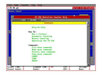
Before commencing a count, ensure the high voltage is set to the correct value by accessing the PRESETS menu bar and selecting the HIGH VOLTAGE function. Others presets such as TIME and COUNT may also be set through this menu.
