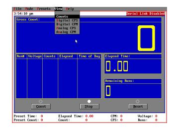
For performing plateau measurements, the high voltage may be set to increase automatically at the completion of each count and the data stored in the Data File. Use the MODE menu to select this feature.
