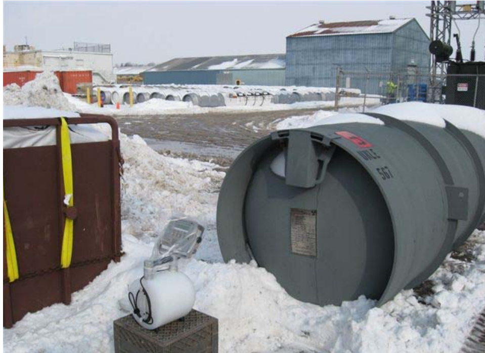
Photograph No. 8: Set up of the Meridian Portable Neutron Monitor 1m from end of test cylinder No. 567. Note storage of cylinders in background. Closest cylinder, which is ready for shipping, is ~30m.
