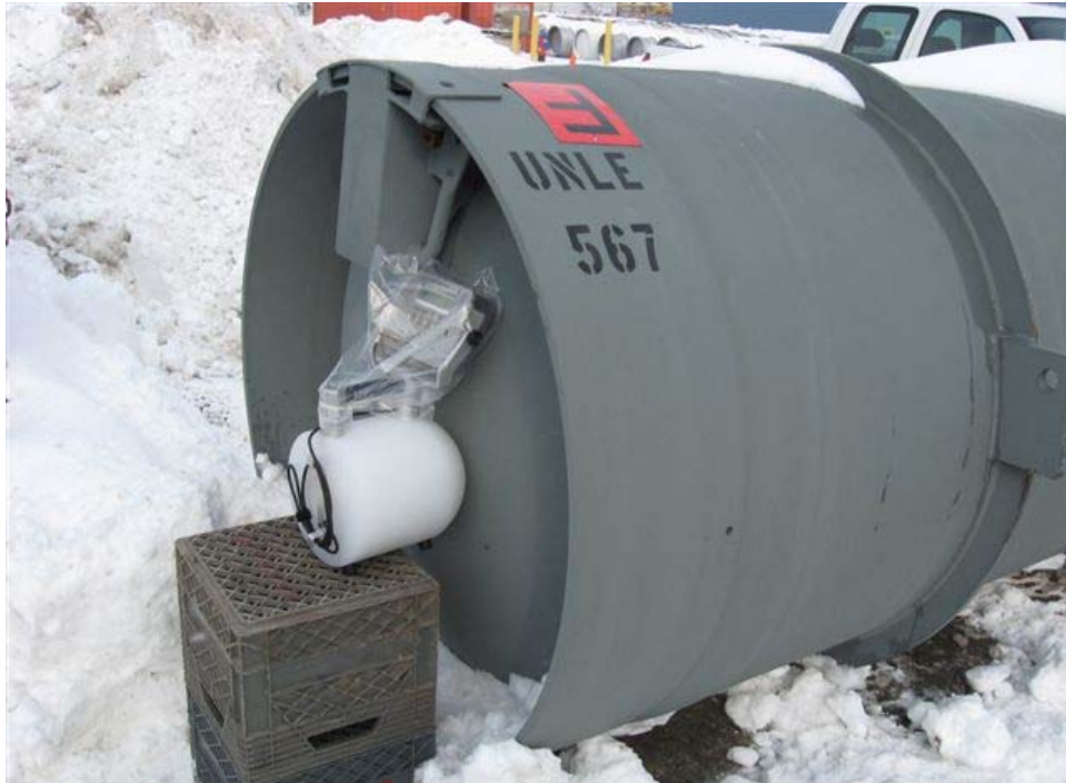
Photograph No. 7: Meridian Portable Neutron Monitor in direct contact with opening end of cylinder No. 567 testing for neutrons.
