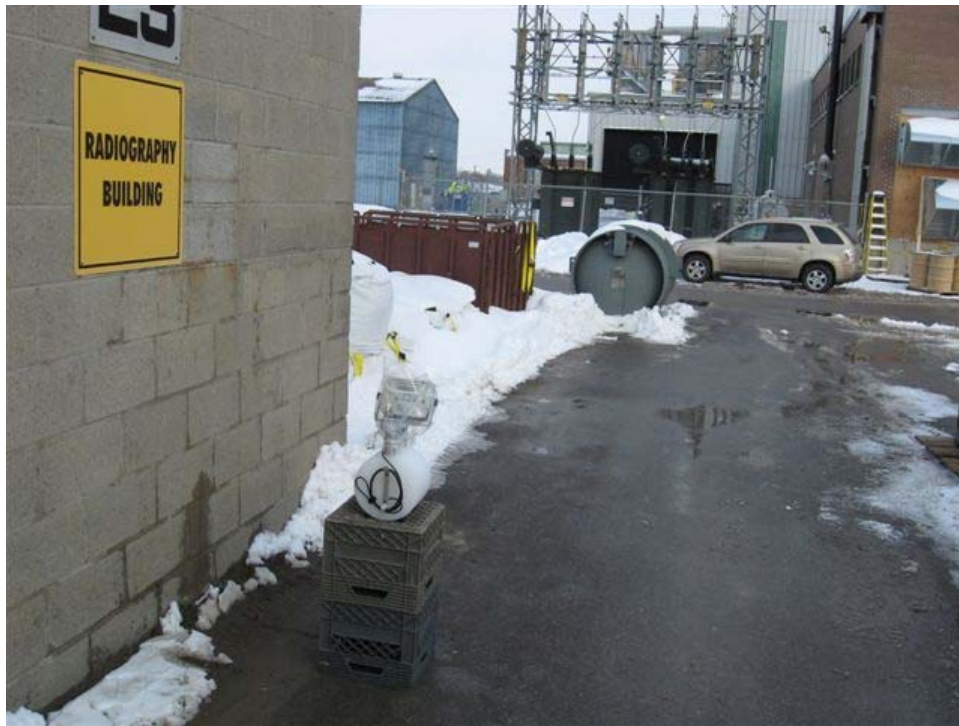
Photograph No. 10: Set up of the Meridian Portable Neutron Monitor 10m from end of test cylinder No. 567.
