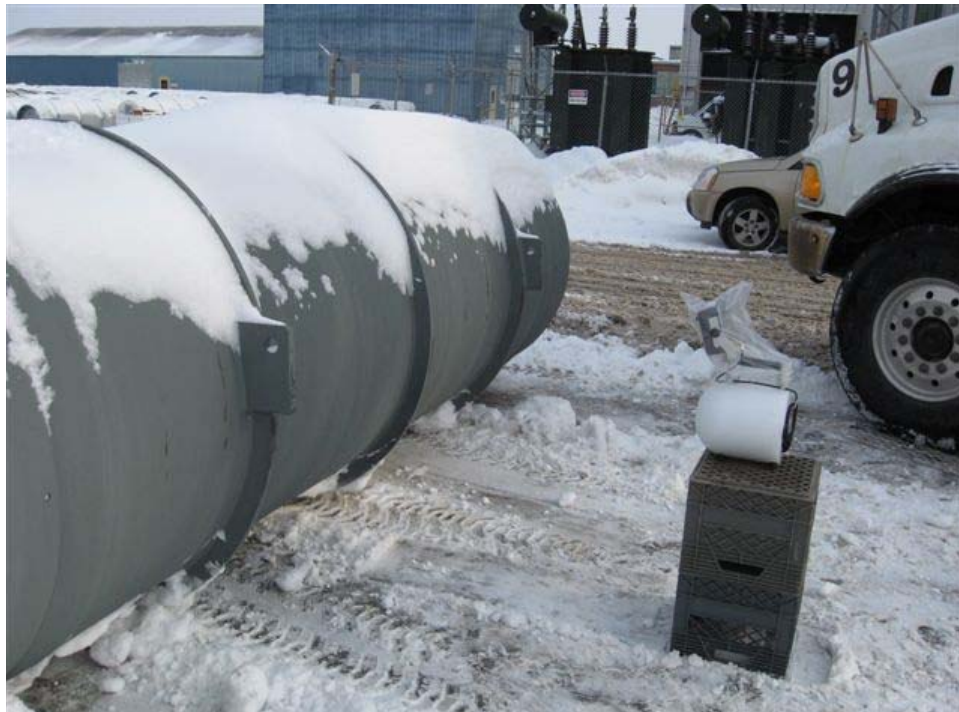
Photograph No. 4: Set up of the Meridian Portable Neutron Monitor 1m from side of test cylinder No. 567.
