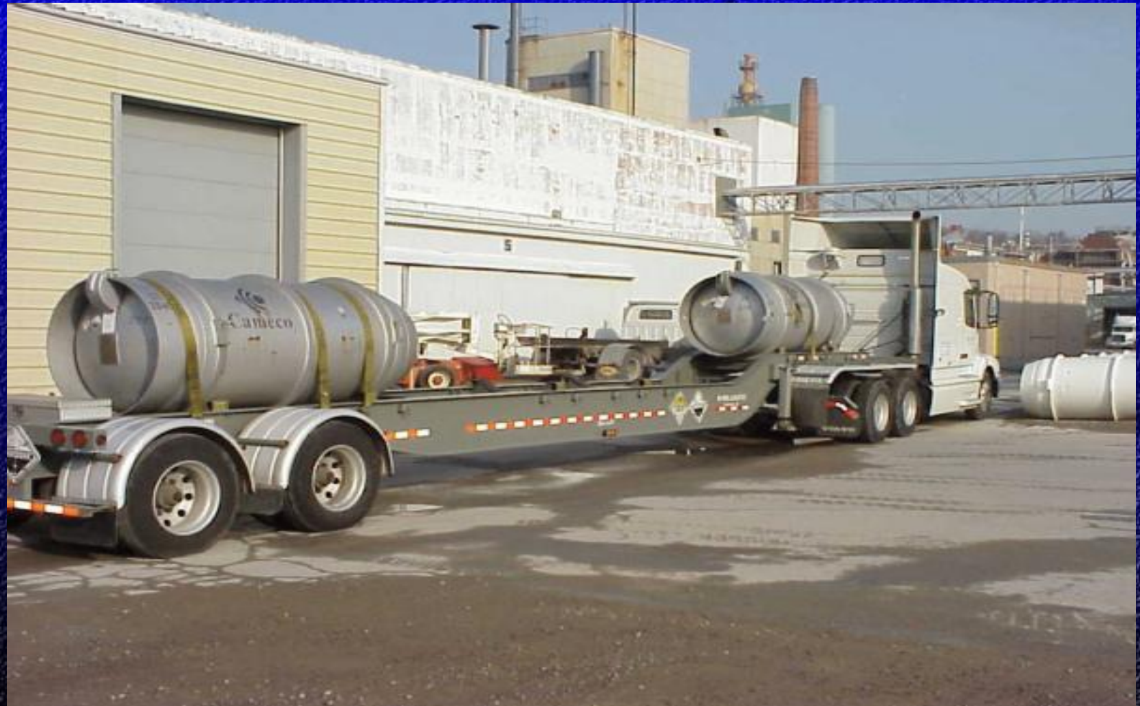
Figure 1. Photograph of open trailer and truck loaded with 2000 48X cylinders for transport to the USA.
