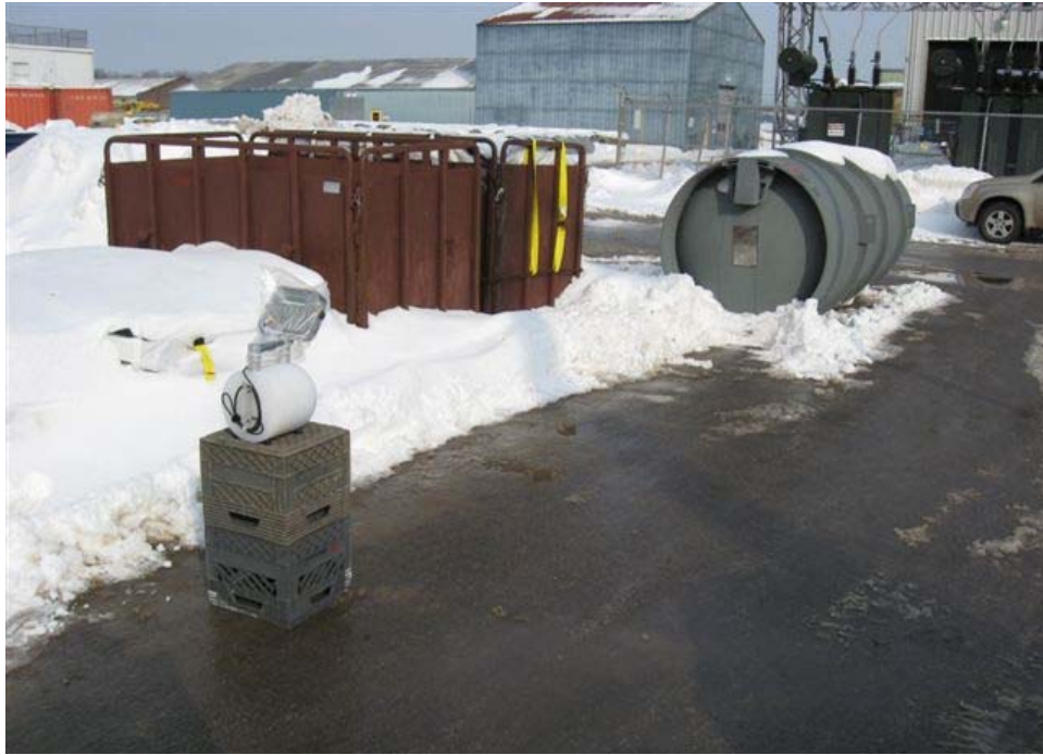
Photograph No. 9: Set up of the Meridian Portable Neutron Monitor 5m from end of test cylinder No. 567.
