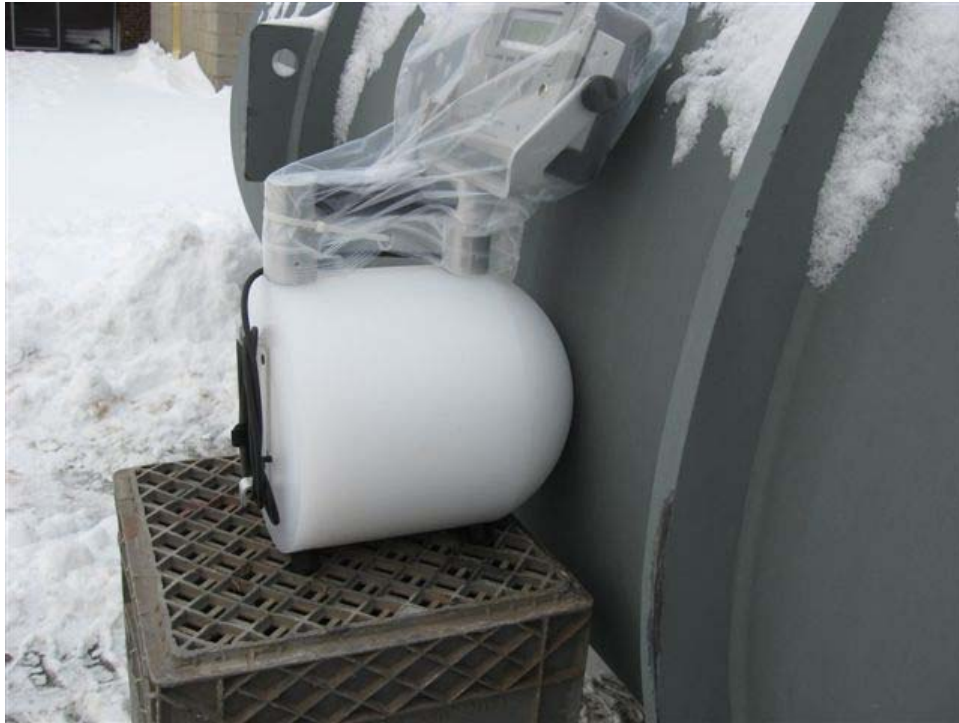
Photograph No. 3: Meridian Portable Neutron Monitor ( Model 5085) in direct contact with side of cylinder No. 567 testing for neutrons.
