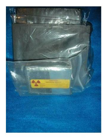
Trying next the HDPE as a reflector, we added one sheet at a time and carefully took readings. More HDPE was better but only up to a point. Fine tuning the reflector resulted in 1 inch as being the most efficient for this neutron energy. Note> In all cases, the source is the same 4" from the He3 tube center. Apparatus is added behind and in front as needed.
