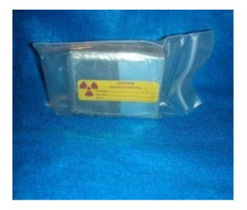
Without any external apparatus, the SAM 935 reads the source as a steady 6 CPM:
