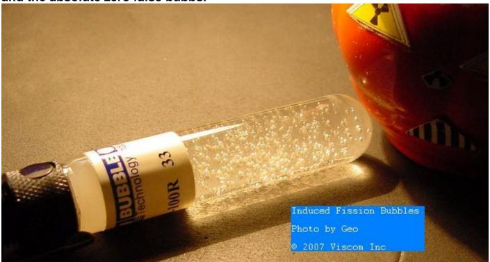
Bubbles captured from exposure to the DU target while it was being bombarded with slow neutrons.
