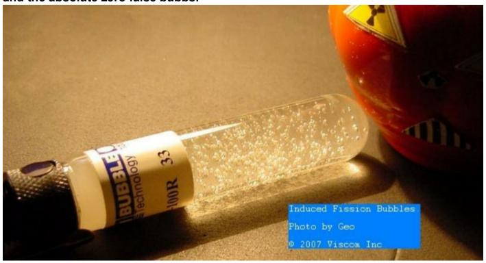
Bubbles captured from exposure to the DU target while it was being bombarded with slow neutrons.
