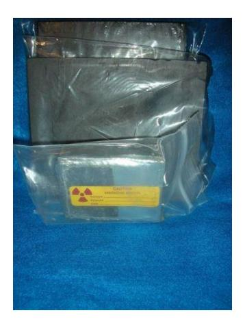
Trying next the HDPE as a reflector, we added one sheet at a time and carefully took readings. More HDPE was better but only up to a point. Fine tuning the reflector resulted in 1 inch as being the most efficient for this neutron energy. Note> In all cases, the source is the same 4" from the He3 tube center. Apparatus is added behind and in front as needed.
