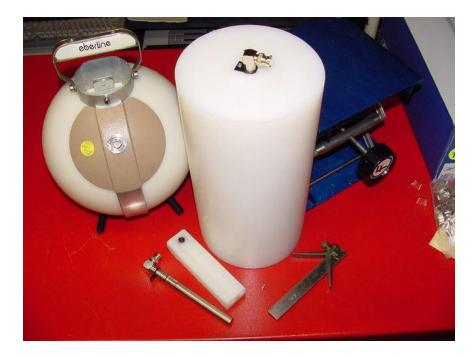
Shown is a very small, temporary Ra/Be neutron source which was constructed for testing purposes then quickly dismantled.
