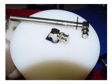
Pictures of home-made neutron detector using 20 atm He3 proportional neutron detector tube. Tube is 1/2" x 4 " active length, He3 is 300 PSI, moderator is 6.5" X 12.5" HDPE. Compare this to the N. Wood BF3 tube in the 9" Remball @ 1" active length. and .78 ATM or roughly equiv. to LND 20126.
