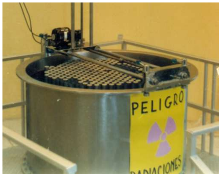
Figure 1.- View of the UAZSNR showing the lattice arrangement.
