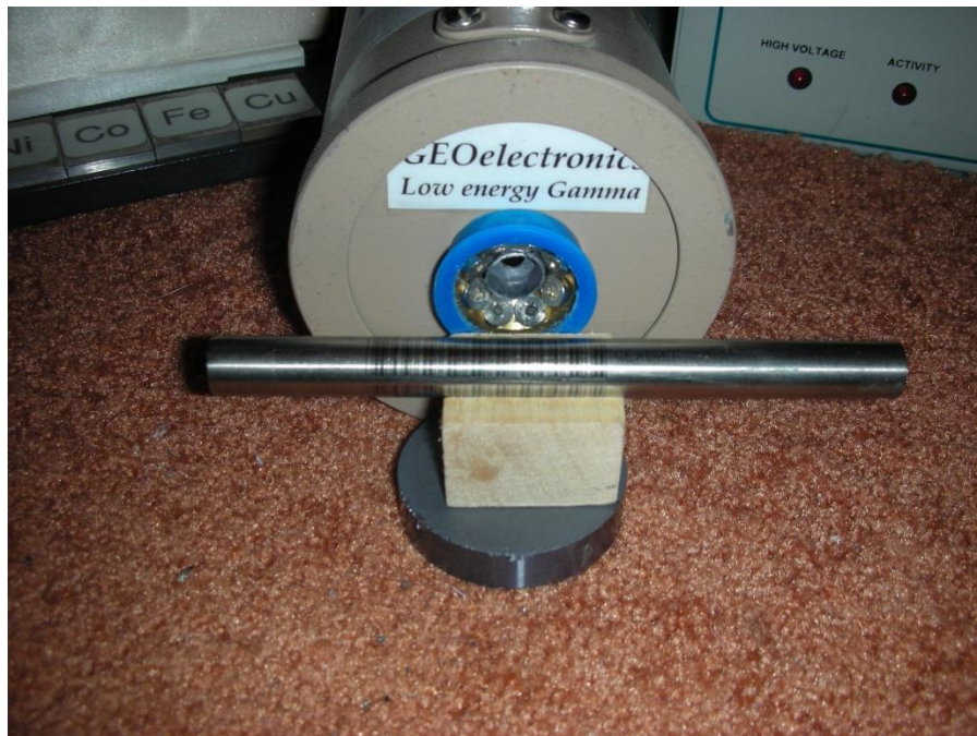
NPP Fuel Rod Cladding Tube- (Zirc4)
