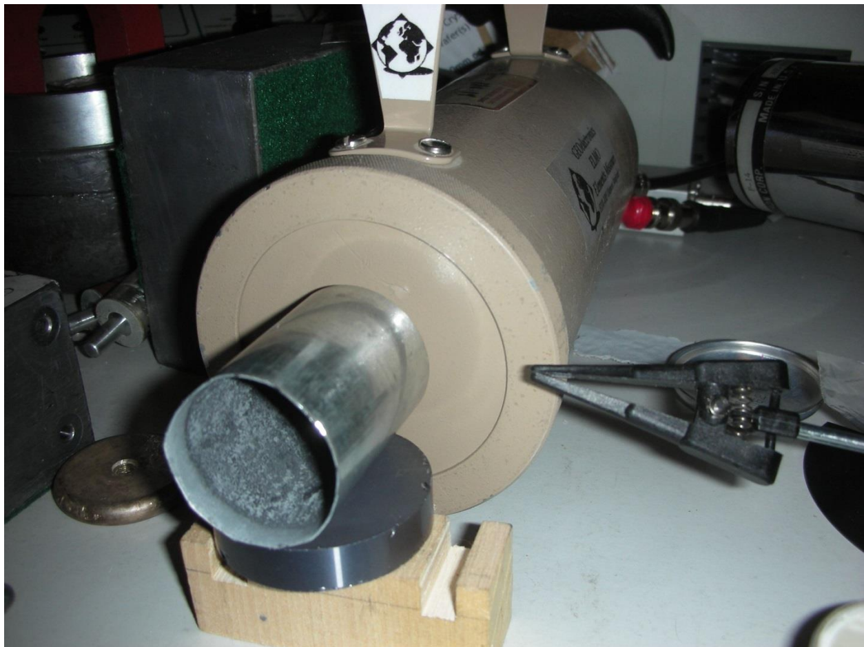
Zinc can, from a carbon-zinc D cell battery
