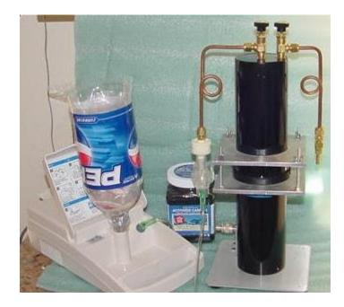
Air is drawn through 40 Th-232 lantern mantles, pulling gaseous Radon 220 (Thoron)
