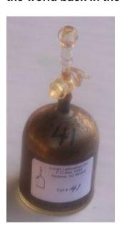
Cells with two valves use a simple air pump to circulate the air, until a sample is collected, when both valves are closed.
