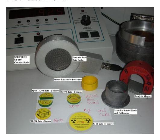
Fig 2: Source holder jig setup. Since we are separating the betas from any other particles or rays that may be coming from the source, we can use mixed-sources, that is one that has multiple types of radiation present. The Cs-137 source is an excellent school lab source, as it has both beta particles and Gamma rays
