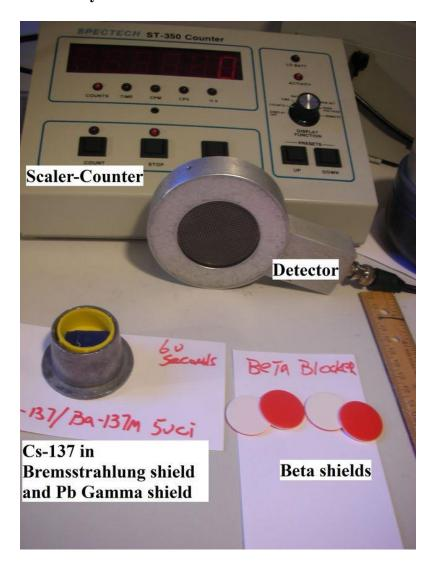
BEFORE EACH TEST, THE ISOTOPE IS PLACED IN THE JIG BUT WITHOUT THE MAGNET. A BASELINE BACKGROUND COUNT IS TAKEN TO DOCUMENT THE BETA SCATTERING ETC.> WITHOUT THE MAGNET PRESENT<.
