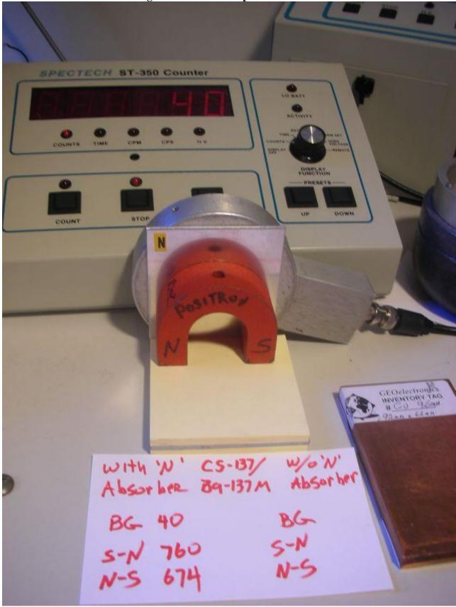
Below is an experiment using TWO DETECTORS (D), (E). One (D) responds to the gamma only from the Cs-137 since gammas
