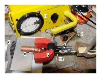
Cs-137 (A) beta-gamma source is shined directly onto the detector (C).
