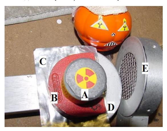
Next is a slightly different setup using an end-window detector which is also sensitive to betas and gammas.
