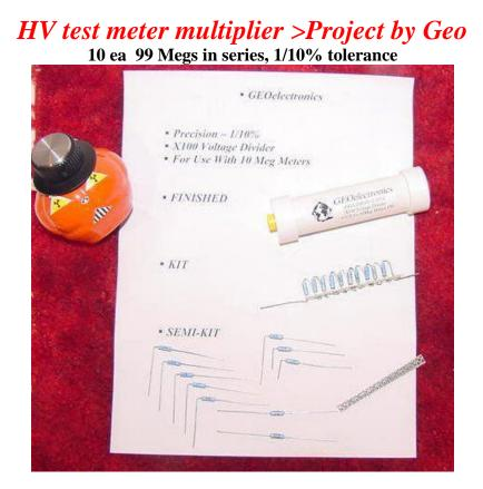
Goes in series with 10 Meg DVM to measure HV in Geiger Counters with precision, without loading down the high impedance circuits. Total 1000 MegOhm including the meter resistance for a X100 multiplication factor on voltages read.
