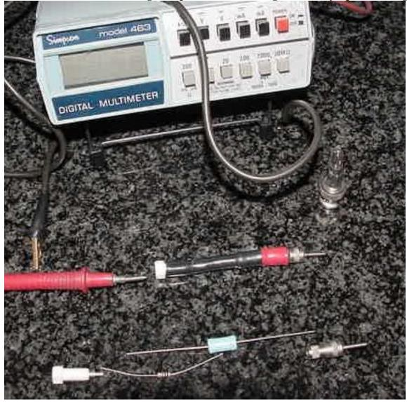
The 1 GigOhm resistor on top of the picture has proved to be quite accurate for our needs when used with a 10 MegOhm input impedance DVM. The bottom resistor is pretty good and much cheaper.
