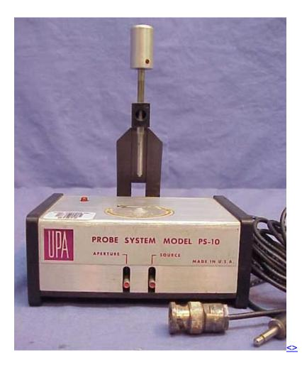
The radioactive source is Pm-147, a beta emitter of 0.2447 MeV (244.7 keV) Peak/ 0.0619 (61.9 keV) keV average at 99.99% probability and a T/2 (Half-Life) of
