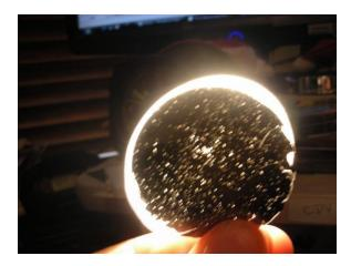
At sea level the mica is slightly bowed inwards due to the reduced pressure of the neon + chlorine gas inside. At higher altitudes, the mica flexes, and at about 8000 feet of altitude or equivalent air pressure, the bow reverses from concave to convex (Passenger airplanes are pressurized to 8000 ft equiv).
