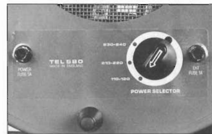
POWER SELECTOR SWITCH AND FUSES LOCATED ON UNDERSIDE OF CABINET.
