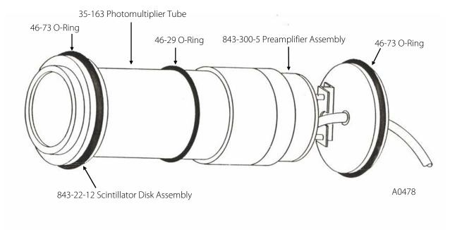
Figure 1-1 Crystal-PM Tube Assembly for Beta Detector 843-22
