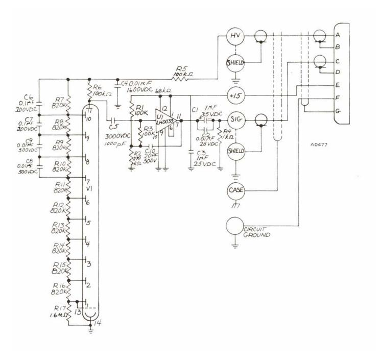
Figure 1-2 Schematic of Preamplifier and PMT for Scintillation Detector 843-22
