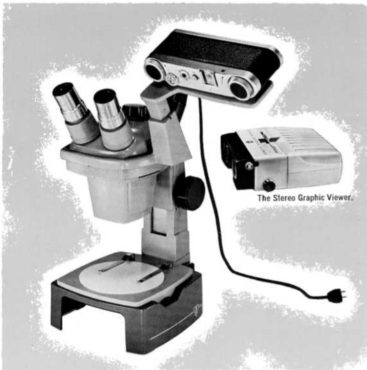
For visual use the camera is swung out of the optical path.
