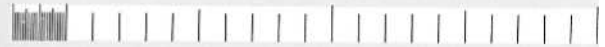
31-16-90 Stage Micrometer for precise calibration of eyepiece discs, 2.2 long, ruled to 0.1mm with 0.2mm ruled to 0.01mm
