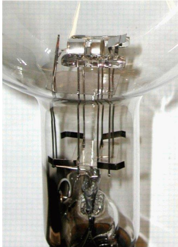
Figure 3: A close-up picture of the e/m electron gun. From this view, the electron beam emerges to the right.
