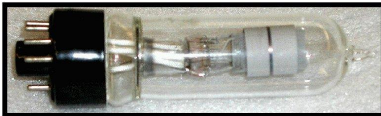
Figure 4: A photograph of a modern Franck-Hertz tube.
