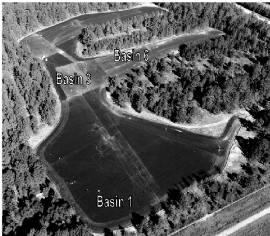
Figure G-10. Aerial photo of the R-Reactors, with seepage basins showing the approximate locations of sampling locations under the asphalt cover installed in 1996
