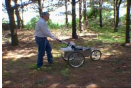
Figure 2-3. Radiation scanning system
