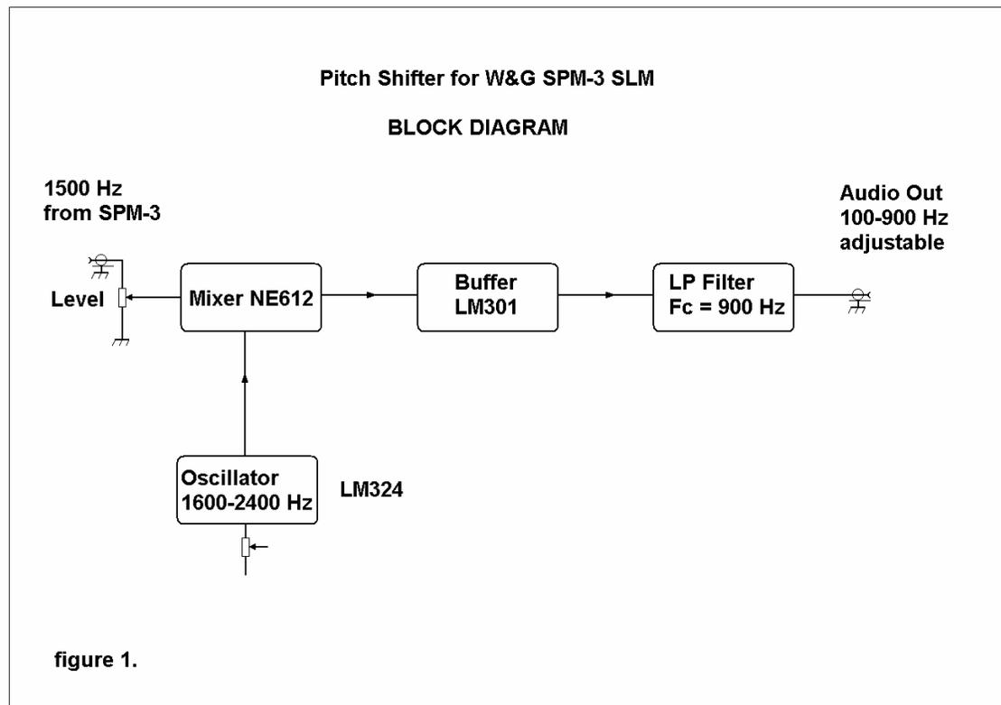
The audio from the SPM-3 or other SLM is fed into the input of a NE612 Gilbert Cell mixer. The Level control adjusts the input level, which is critical for lowest distortion. A separate Wien Bridge Oscillator generates the required signal to convert the 1500 Hz. The output pitch is dependant from the frequency of the oscillator. The beat note can be set to any frequency in the 100 – 900 Hz range.
