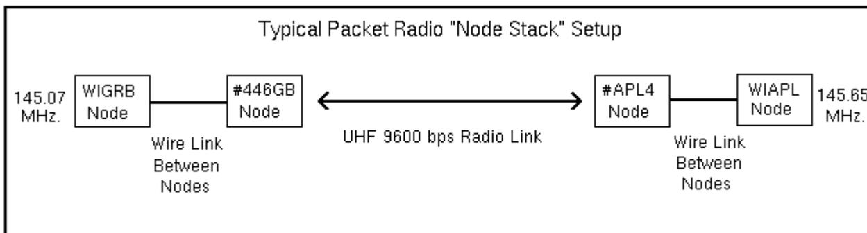
If you guessed that the people operating on the Green Bay LAN can connect to the people operating on the Appleton LAN even though they are on different frequencies, you are right. Other LANS can be arranged so that they, too are on the backbone. This is the basis of a packet radio network. In the next part of this series, we will put this knowledge to work. We'll use information you can get from a node in order to explore the network.
