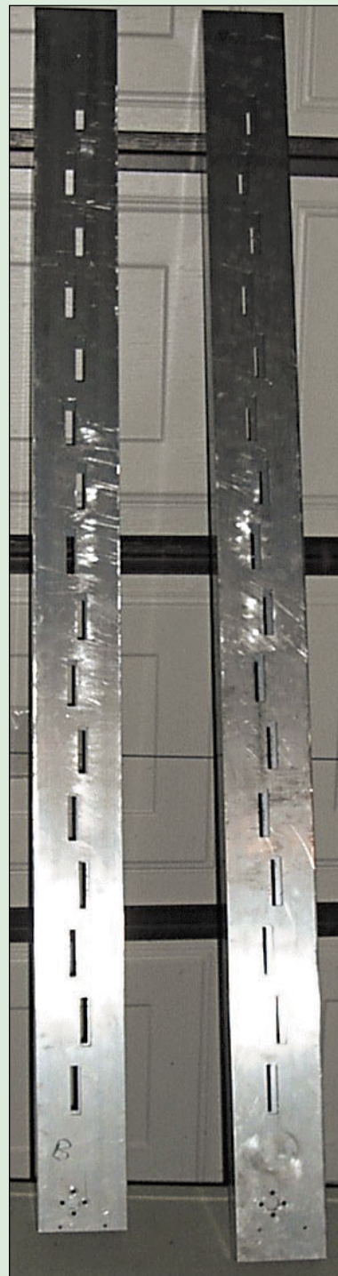
Figure A—The design of the slot antenna allows it to be easily reproduced with a milling machine.
