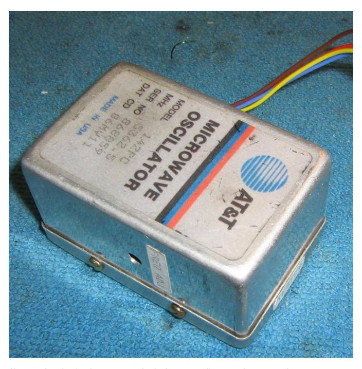
Alternate view showing the access port for the frequency adjustment trimmer capacitor.
