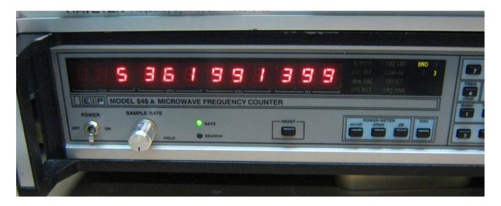
Tweaking the oscillator's final output frequency down to 5362.0 MHz, or as close as possible.
