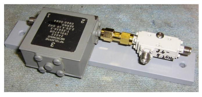
An optional ferrite isolator and a 20 dB directional coupler are added to RF output of the amplifier.
