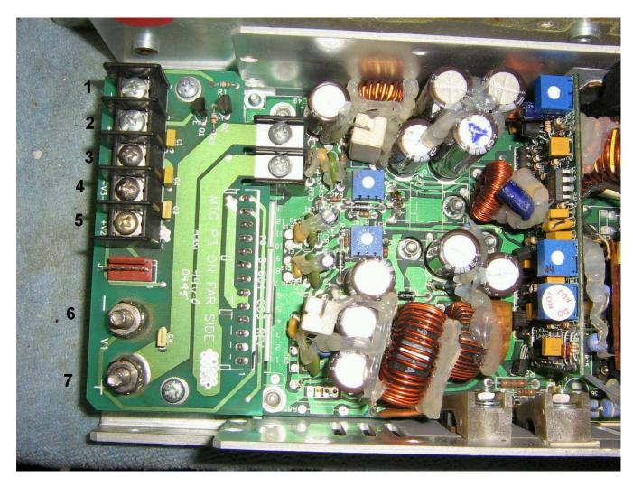
Closeup view of the Xentek's power supply's output terminals.
