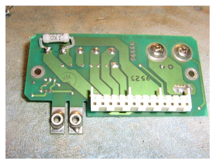
1k ohm / 3 watt load resistor across the +24 VDC output.
