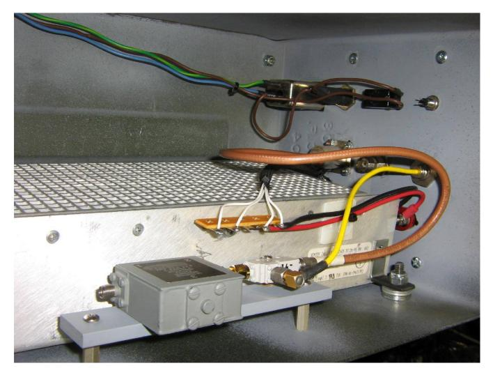
Mounting the ferrite isolator and directional coupler.
