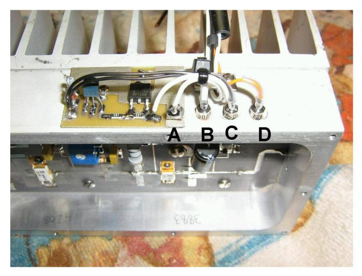
Closeup view of the negative voltage sequencer circuit board and the amplifier's DC power connections.
