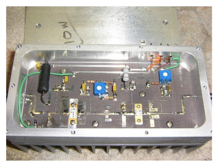
Internal view of the Comwave 10 watt MMDS amplifier.
