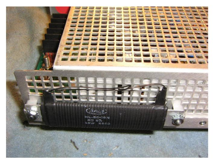
5 ohm / 55 watt load resistor across the +5 VDC output.
