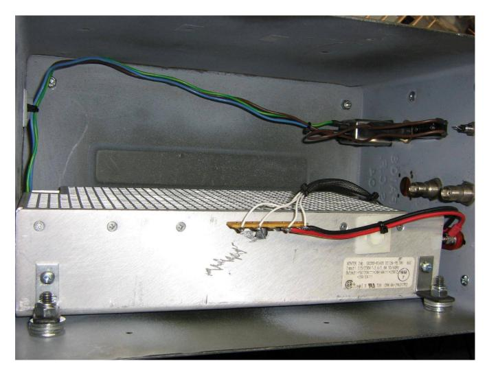
Mounting the switching power supply inside the project case.
