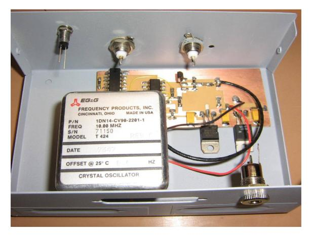
Mounting the oscillator and circuit board.
