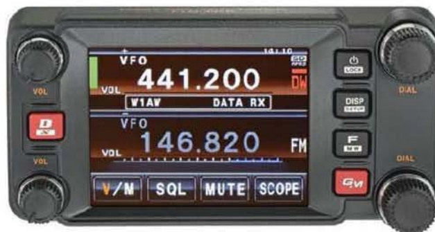
Figure 2 — The FT-400DR set up for full rate data communication on Band A (top) and analog FM voice on Band B. There are independent volume controls and dial knobs for each band. The functions of the buttons along the bottom of the touchscreen can be changed by the user.
