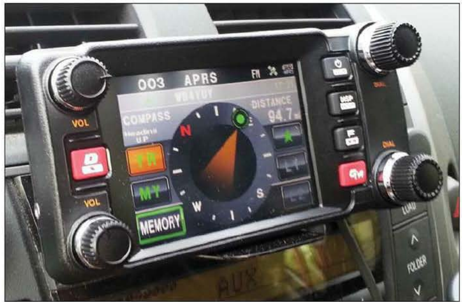
Figure 1 — The FTM-400DR control head with its mounting bracket inserted into the CD player slot in the author's dashboard. The display is showing the bearing and distance to an APRS station.
