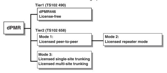
As the diagram shows, dPMR<sup>™</sup> is a full featured system capable of providing communications solutions ranging from license-free all the way up to nation-wide networks. The main difference to NXDN<sup>™</sup> is additions of the license-free standard. The dPMR<sup>™</sup> protocol allows for system sizes up to a potential of 1,000 sites and millions of users.
