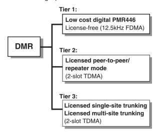
As the diagram shows, DMR is also a full featured system capable of providing communications solutions ranging from license-free all the way up to nation-wide networks.
