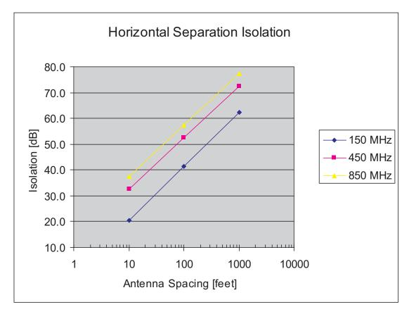
Figure A-3 Horizontal Separation Isolation
