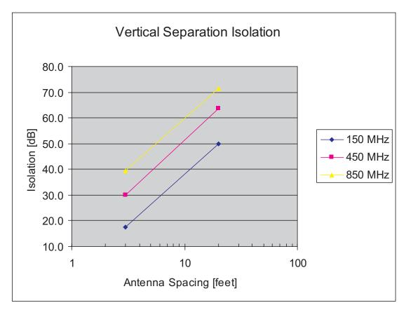
Figure A-4 Vertical Separation Isolation
