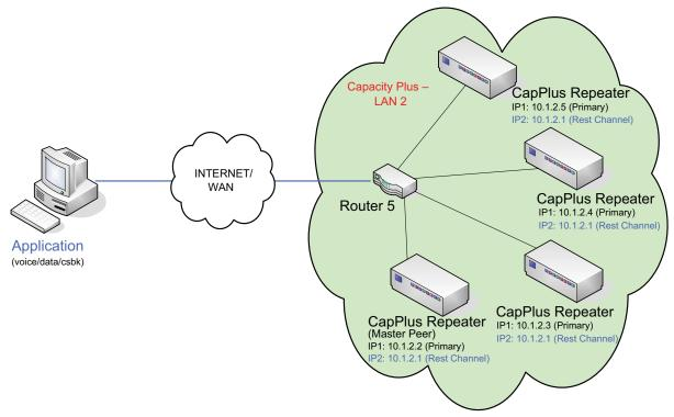
Figure 2-28 Capacity Plus System with IP-based ADP Application
