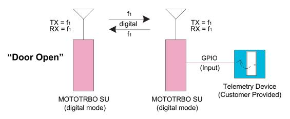
Figure 3-10 Send Telemetry Message from MOTOTRBO Radio to Another MOTOTRBO Radio when Input Pin State Changes
