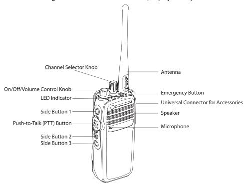
Figure 3-3 MOTOTRBO Portable (Non-Display Model)
