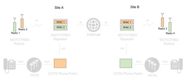
Figure 2-23 Two APP Boxes Supporting Two Wide Area Channels in IP Site Connect
