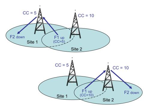
Figure 4-15 Multiple Digital Repeaters with Unique Color Codes
