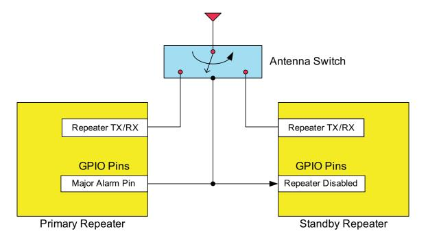
When a major alarm happens three times in the primary repeater and the repeater enters the locked state, the primary repeater will set the major alarm GPIO pin to active level. The standby repeater detects the disable pin is changed to inactive level and it becomes enabled. The antenna switch is also triggered which changes the antenna to the now active repeater.
