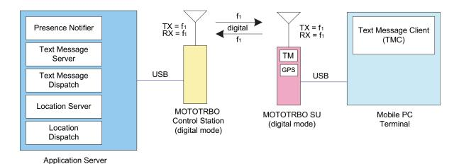
Figure 3-13 MOTOTRBO Radios In Digital Direct Mode with Text Message Server, Location Server and Local Dispatchers
