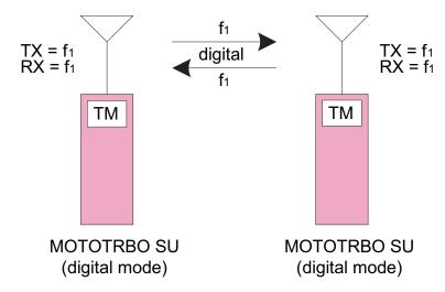
Figure 3-7 MOTOTRBO Radios (in digital mode) Text Messaging In Direct Mode
