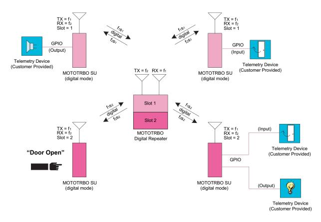
Figure 3-22 MOTOTRBO Radios in Digital Two-Slot Digital Repeater Mode with Telemetry Functions
