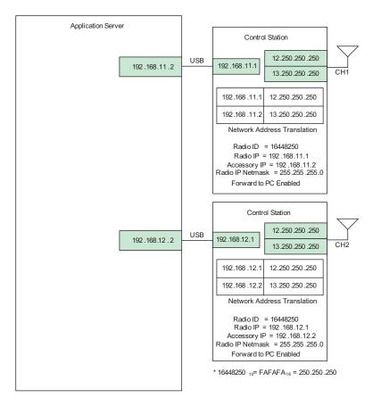
Figure 4-24 Application Server Control Station Network Connectivity
