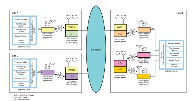
Figure 3-34 Wide and Local Area System with Distributed Data Application Servers
