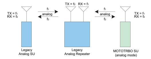
Figure 3-30 MOTOTRBO Analog and Legacy Analog Radios on Legacy Analog Repeater
