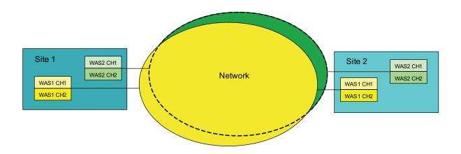
Figure 2-14 Two Wide-Area Systems, Each with Two Wide-Area Channels
