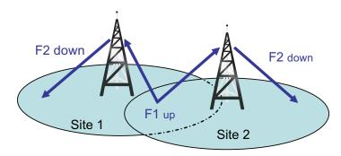
Figure 4-14 Multiple Repeaters with Overlap and Common Frequencies
