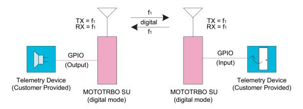
Figure 3-11 Send Telemetry Command to Toggle an Output Pin from MOTOTRBO Radio to Another MOTOTRBO Radio when Input Pin State Changes
