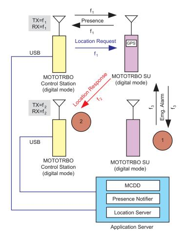
Figure 4-27 Emergency Alarm and GPS Revert Interaction Diagram
