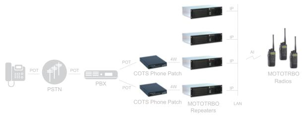
Figure 2-25 Phone Patch Topology in a Capacity Plus Configuration
