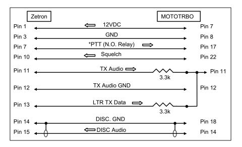
Figure 2-26 DR 3000 Cable Schematic for Zetron Controllers
