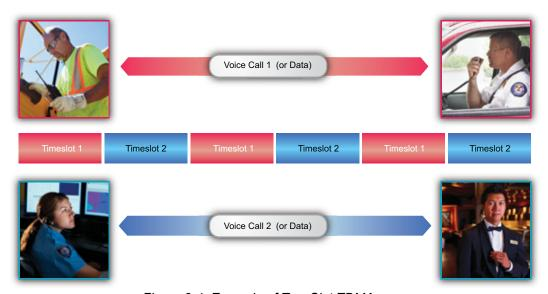
Figure 2-4 Example of Two-Slot TDMA
