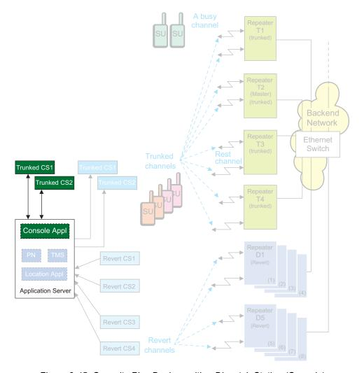
Figure 3-45 Capacity Plus Devices with a Dispatch Station (Console)
