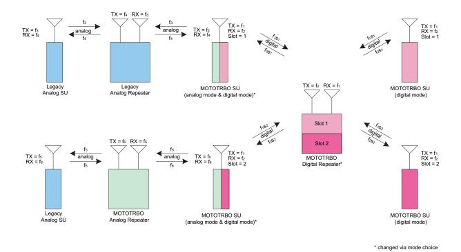
Figure 3-32 MOTOTRBO Digital Radios on a Two-Slot MOTOTRBO Digital Repeater with Analog Legacy
