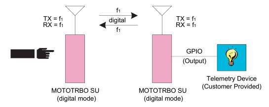
Figure 3-9 Send Telemetry Command from MOTOTRBO Radio to Another MOTOTRBO Radio to Toggle an Output Pin
