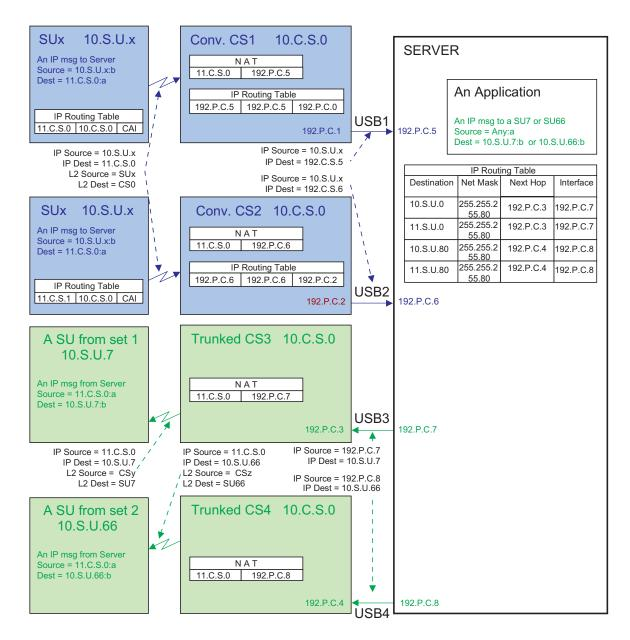
Figure 4-26 An example showing IPv4 addresses in a Capacity Plus configuration with Data Revert
