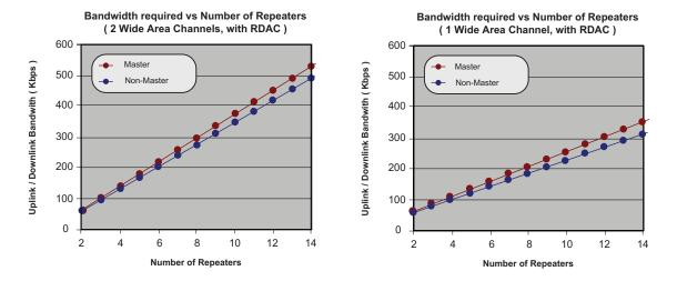
Figure 4-18 Required Bandwidth for Two Simple IP Site Connect System Configurations
