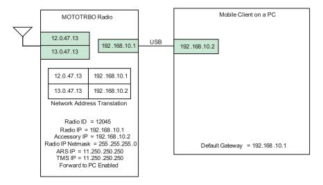
Figure 4-23 Air Interface Network Connectivity
