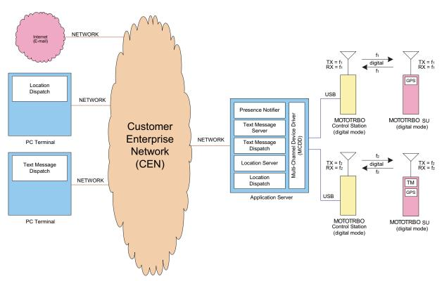
Figure 3-15 MOTOTRBO Radios in Two Channel Digital Direct Mode Server-Based Configuration with Remote Dispatchers
