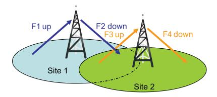
Figure 4-13 Multiple Repeaters with Overlap
