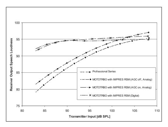
Figure 2-7 Transmit Audio Sensitivity
