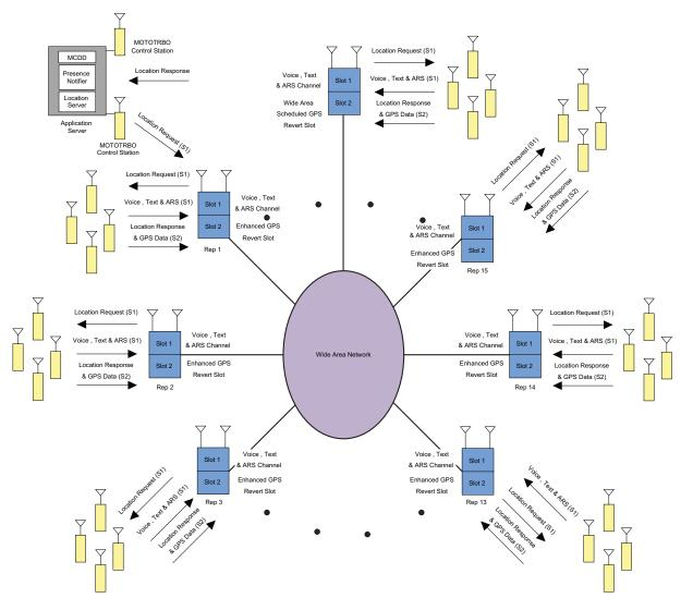
Figure 3-28 IP Site Connect System with an Enhanced GPS Revert Channel
