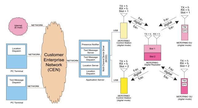
Figure 3-24 MOTOTRBO Radios in Digital Two-Slot Digital Repeater Mode with a Server-Based Configuration and Remote Dispatchers
