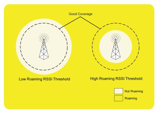
Figure 2-15 Roaming Triggered by Roaming RSSI Threshold Value
