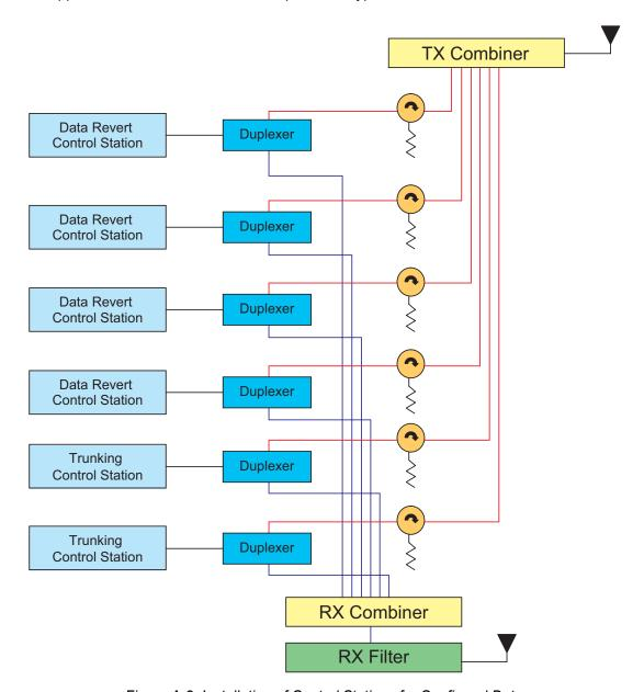
Figure A-2 Installation of Control Stations for Confirmed Data
