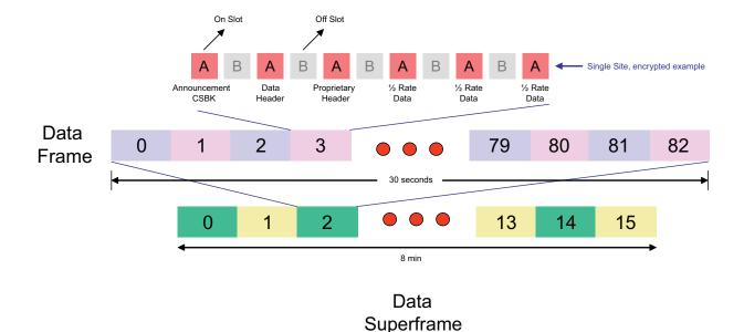
Figure 2-10 Windowed Data Structure for a Window Size of Six
