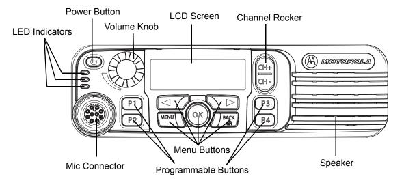
Figure 3-4 MOTOTRBO Mobile Control Head (Full Display Model)
