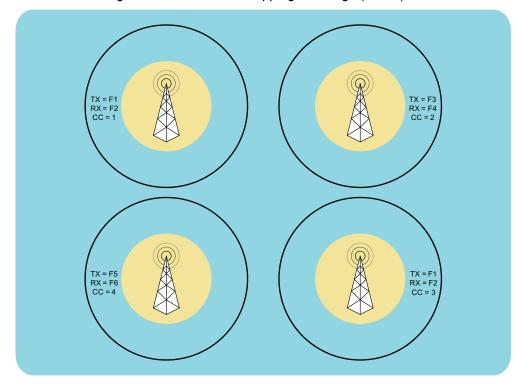
Figure 2-17 Isolated No Overlapping Coverage (Rural)
