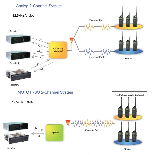
Figure 2-3 MOTOTRBO Requires Less Combining Equipment
