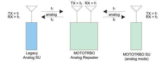
Figure 3-31 MOTOTRBO Analog and Legacy Analog Radios on MOTOTRBO Analog Repeater
