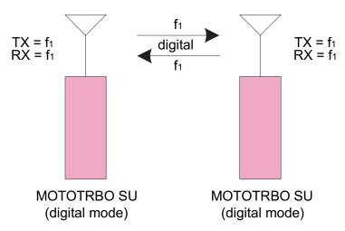
Figure 3-6 MOTOTRBO Radios (in digital mode) In Direct Mode
