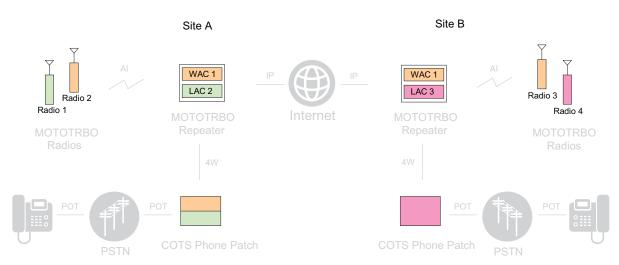
Figure 2-24 APP Boxes Supporting Wide Area Channels and Local Area Channels in IP Site Connect
