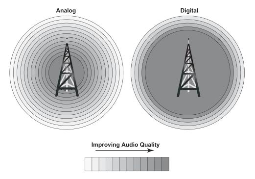
Figure 2-6 Differences in Analog Coverage
