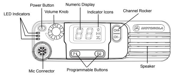
Figure 3-5 MOTOTRBO Mobile Control Head (Numeric Display Model)
