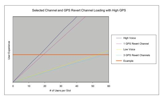
Figure 4-6 Channel Loading with GPS Revert Channels
