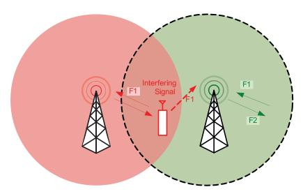
Figure 4-20 An Example of Interference at Receive Frequency
