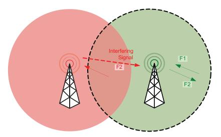
Figure 4-21 An Example of Interference at Transmit Frequency
