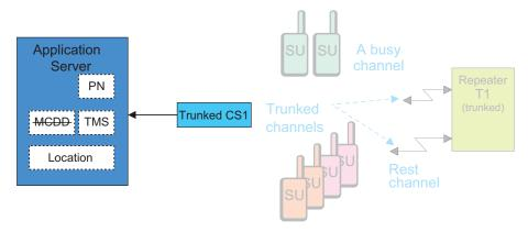
Figure 3-43 Two-channel Capacity Plus Devices with Data over Trunked Channels
