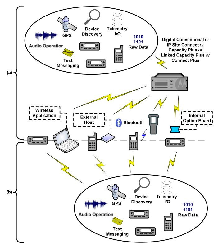
Figure 4-3 Interoperability Examples of Radio Control Solution Topologies – (a) MOTOTRBO Digital System-based and (b) MOTOTRBO Digital Talkaround
