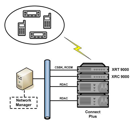
Figure 4-5 Typical Network Management Solution Topology Example for Controller-based Systems
