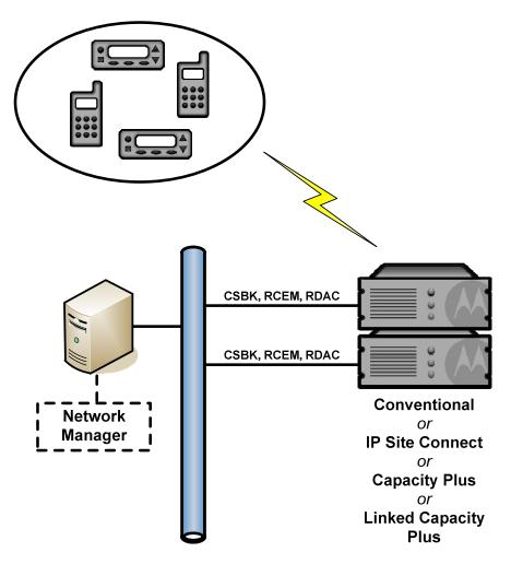
Figure 4-4 Typical Network Management Solution Topology Example for Controller-less Systems
