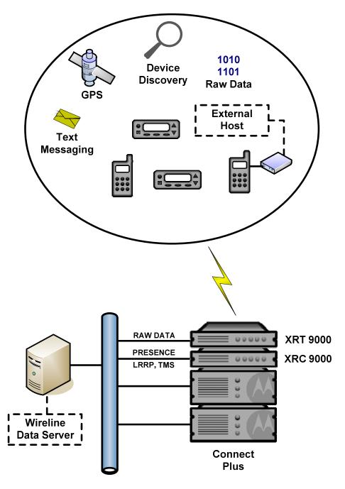
Figure 4-2 Typical Data Server Solution Topology Example for Controller-based Systems – Wireline Data Server
