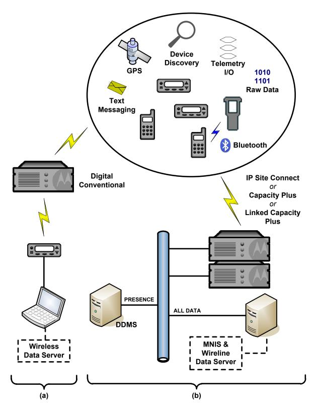
Figure 4-1 Typical Data Server Solution Topology Examples for Controller-less Systems –
