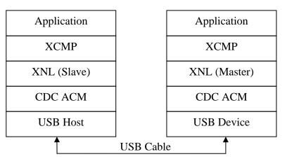
Non-IP Capable Peripheral MOTOTRBO Radio
