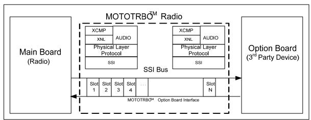
Figure 2 - MOTOTRBO™ Option Board Interface Architecture
