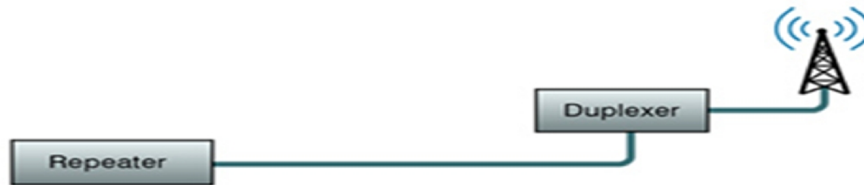
Repeater Equipment for Two Channel DMR
