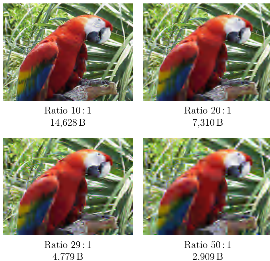
Figure 9.7: File size depends on the compression ratio of JPEG 2000.
