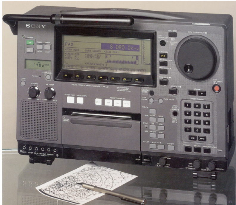
Figure 11.4: Modern receiver Sony CRF-V21 for WEFAX and RTTY reception equipped with printer.
