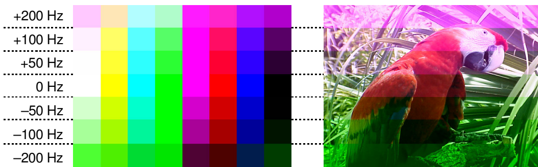
Figure 3.9: Color distortion of YCrCb when the station is improperly tuned.
