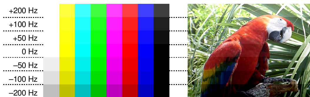
Figure 3.10: Color distortion of RGB when the station is improperly tuned.
