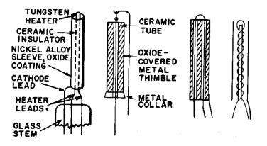
**FIGURE #4: Cathode Structure:**
