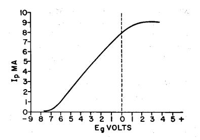
Figure. #15. Typical Eg - Ip Characteristic curve:
