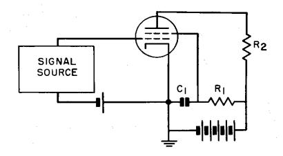
Figure. #24. Schematic of a screen grid amplifier circuit:
