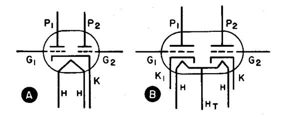
Figure. #27. Dual triode tubes. The tube at "A" has a common cathode. The tube at "B" has two separate cathodes. Notice this tube has a single heater with a center tap. Not all tubes of this type have tapped heaters.
