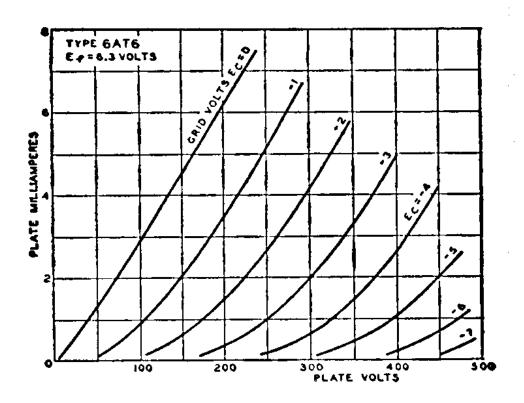
Figure. #20. EP-IP curves of " a 6AT6 tube.
