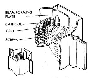
Figure. #25. A beam-power tube structure:
