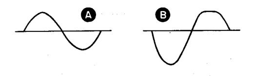
Figure. #16 A/B: Input voltage = "A" and output voltage = "B" The flattened top on the right side of the "B" waveform is distortion from access bias:
