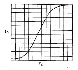
Figure. #6: Diode Characteristic Curve: The characteristic curve of a diode showing the relationship between plate current and plate voltage. Notice that there is a small plate current even when the plate voltage is zero. This is caused by a few electrons being emitted by the cathode at such a high speed that they travel over and strike the plate even when no voltage is applied to it.
