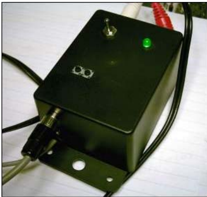
Left: The outside view of the box I mounted my SGC module in. You can see the small push buttons near the lower left-hand side. The green LED shows that the power is on, and the switch is a DPDT type for bypassing the unit.
