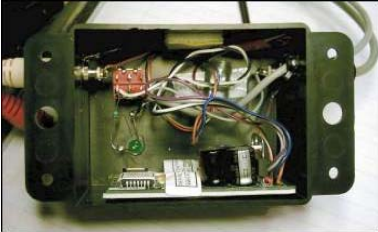
Left: The SGC module seen here mounted inside an ABS plastic box.
