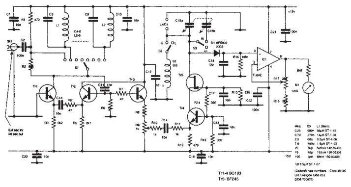
**Figure 4.9** The switched frequency rf source ( $Tr_1$  to  $Tr_3$ ) provides a constant level drive source to the reactance under test, and detector/measurement circuit  $D_1 IC_1$ . NOTE:  $R_1$  is 47 $\Omega$ , 47R resistor at  $C_{13}$  is  $R_4$ , emitter follower at  $R_8$  is  $TR_3$
