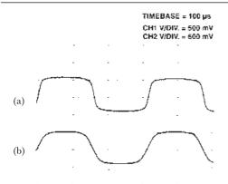
**Figure 2.2** (a) Smoothness of square waveform across V<sub>d</sub>. (b) Connecting R<sub>11</sub>, 33 k $\Omega$  in parallel with the diodes results in more gently sloping sides
