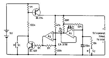
**Figure 6.4** Analog delay circuit avoids possibility of interference from oscillator.  $A_1$  and  $A_2$  are CA3130
