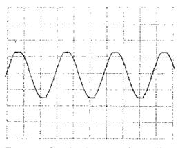
**Figure 2.5** Showing the output of an oscillator to the design of Figure 2.4
