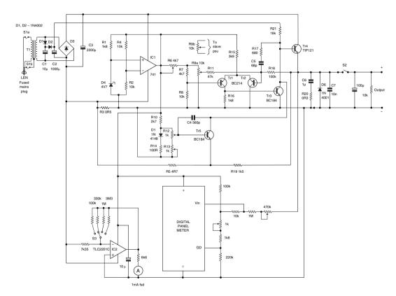
**Figure 6.28** Full circuit diagram of the versatile power supply, including the analog current meter circuit. Components shown are for a 15 V, 1 A output, but the circuit is easily altered for other outputs
