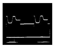
**Figure 5.4** Device operating in the circuit of Figure 5.3. Lower trace: SI pulses; upper trace: analog output at  $A_o$  with part of the line array covered
