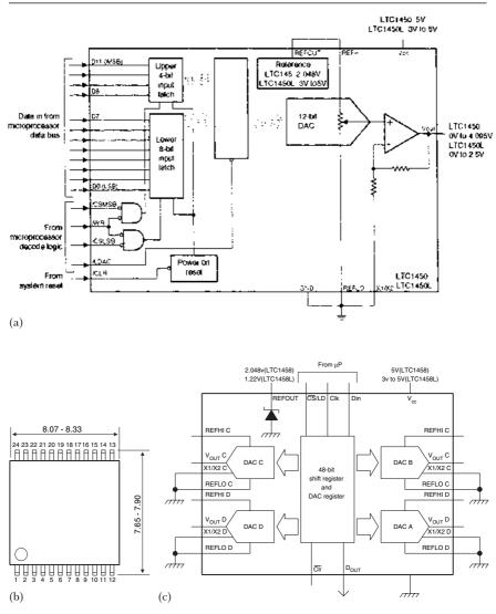
**Figure 1.34** The LTC1405, (a), from Linear Technology is a 12 bit DAC with parallel data input. This requires a 24 pin package, (b), but the Small Outline pack is still much smaller than the corresponding DIP. (c) shows a block diagram of the internal workings of the LTC1458, from the same manufacturer. This quad DAC comes in either an SO pack, or the even smaller SSOP, both with 28 pins, achieved by using a 48 bit serial data input stream
