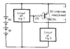
of a milliamp) would one want to leave it permanently connected across the battery. Figure 6.8 shows how it can be adapted for use with the stabilised delay switch-off circuit of Figure 6.7. The 22 k $\Omega$  pot would of course be set to indicate a battery end voltage of 12.5 V.
