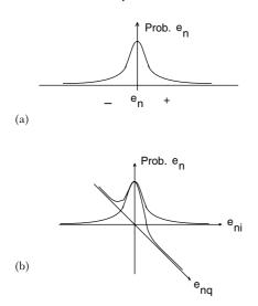
**Figure 7.28** (a) Voltage probability distribution of a real signal (same as Figure 7.24). (b) Voltage probability distribution of the in-phase and quadrature components of a narrowband noise (a complex signal)
