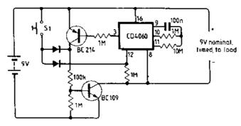
**Figure 6.3** Delay circuit using an oscillator, followed by a counter. Very long delays can be obtained by this method
