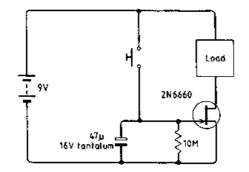
**Figure 6.2** VMOS circuit, which is simple but which does not turn off cleanly
