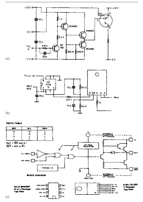
**Figure 6.13** (a) Useless gate driver circuit Mark 1. (b) Gate driver circuit using the Unitrode UC3705N. (c) Internal circuit
