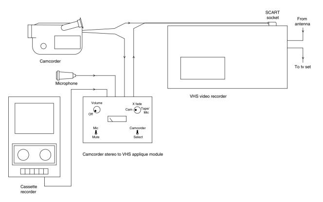
**Figure 2.26** Showing the various pieces of kit interconnected. The sound from the camcorder is routed via the appliqué box. The latter permits cross-fading of the camcorder sound output with sound from tape and/or microphone
