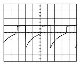
**Figure 5.28** *Light output of the circuit of Figure 5.27, measured using range 4 of the light-meter, at a range of 1 cm. 500 mV/div.vertical, 0 V reference line at one division above centreline, 10 µs/div. horizontal*
