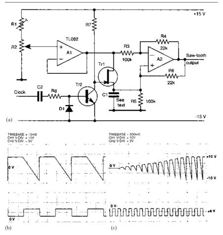
**Figure 4.12** (a) Basic circuit of the tuning sweep generator, employing a Howland current pump ( $A_2$  and associated resistors). (b) Output waveform shown in relation to the controlling clock waveform. (c) Advancing  $R_2$  from ground to maximum increases the sweep width whilst remaining ground-centred
