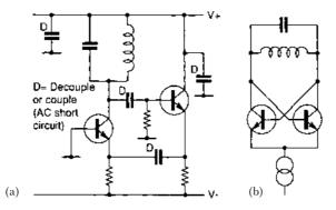
**Figure 4.8** (a) Two transistor oscillator looks at first sight like an emitter follower driving a grounded base stage. But the earth point is an arbitrary convention. (b) If the decoupling capacitors in (a) are shown as short-circuits at rf, the circuit is seen to be a balanced push–pull oscillator
