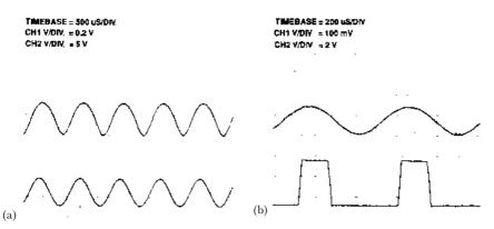
**Figure 7.18** (a) The TXM-UHF and SILRX-418-A can handle linear signals, with some distortion; 1 kHz full amplitude sinewave modulation applied to TX module (lower trace) and as recovered by the receiver (upper trace). (b) At a reduced modulation level (upper trace) the distortion of the received signal is negligible, although the effect of a reduced level into the data slicer is evident (lower trace)
