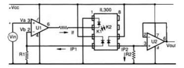
**Figure 5.10** Typical application circuit for the IL300 linear optocoupler, in positivegoing unipolar photoconductive model. Although K<sub>1</sub> and K<sub>2</sub> vary with temperature, their ratio K<sub>3</sub> is virtually temperature independent. Devices are coded into bands according to the spreads of K<sub>1</sub> and K<sub>3</sub>
