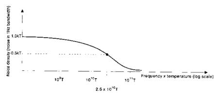
**Figure 7.21** The level of thermal 'white' noise falls off above a certain frequency which depends upon the temperature
