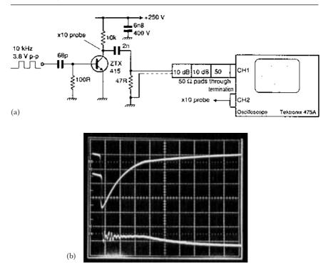
**Figure 1.13** (a) Test set-up used to view the pulse produced by an avalanche transistor. (b) Upper trace, voltage across load, effectively 50 V/div. (allowing for 20 dB pad), 0 V = 1 cm down from top of graticule, 50 ns/div.; lower trace, collector voltage, effectively 50 V/div. (allowing for ×10 probe), 0 V = 1 cm up from bottom, 50 ns/div.
