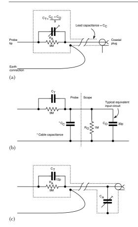
**Figure 3.25** (a) Circuit of traditional 10:1 divider probe. (b) Equivalent circuit of probe connected to oscilloscope. (c) Modified probe circuit with trimmer capacitor at 'scope end
