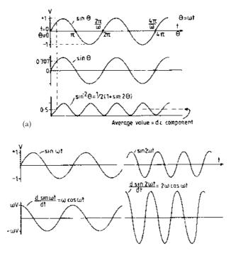
**Figure 7.6** Effects of squaring and differentiating sine waves. Squaring the wave, as in (a), doubles its frequency and produces a dc component. Differentiating, shown in (b), gives a cosine wave with an amplitude proportional to frequency
