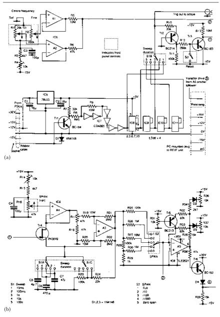
**Figure 4.13** (a) Sweep duration generator and centre-frequency setting circuits. (b) Sweep generator, sweep/centre-frequency summer and sweep shaping circuits. NOTE:  $C_6$  and  $C_7$  are 470n and 47n respectively
