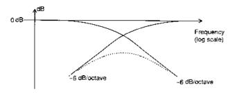
**Figure 2.20** *Cascaded lowpass and highpass* CR *responses, and their resultant,* (dotted)
