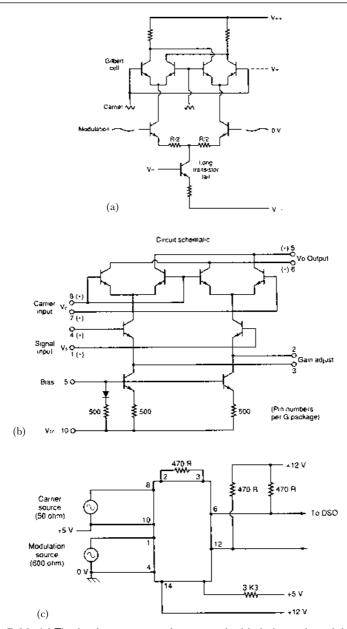
**Figure 7.11** (a) The basic seven transistor tree double balanced modulator. (b) An *IC* version is available from many manufacturers under type numbers such as LM1496, LM1596. Note that pin numbers refer to the round G package. (c) Simple test circuit using LM1496. Note that pin numbers refer to the DIL P package
