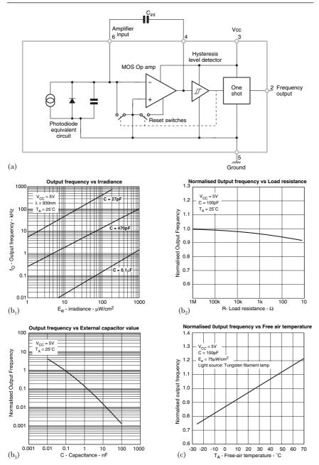
**Figure 5.20** (a) Internal workings of the TSL220. (b) Output frequency of the TSL220 versus incident illumination for various values of capacitor, top left, with load and normalised capacitance curves. (c) Output frequency versus temperature, normalised to 25°C, of the TSL220 under the stated conditions
