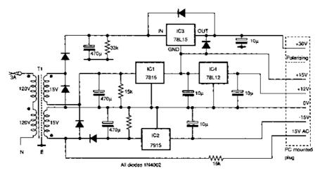
**Figure 4.11** Stabilised power supplies. Nominal 15 V secondaries produce 22 V dc raw supplies. The 15 V ac output provides a timebase for the sweep voltage generator
