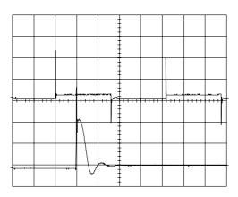
**Figure 6.22** Transient response of the PSU when the load switches between 0.5 A and 1 A: upper trace 200 mV/div., 200 µs/div.; lower trace 200 mV/div., 5 µs/div.
