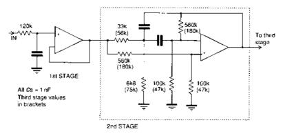
**Figure 2.25** A 5 pole elliptic filter with 0.28 dB passband ripple and an attenuation of 54 dB at 1.65 times the cut-off frequency and upwards. The –3 dB point is 3 kHz, approx. All capacitors C = 1 nF, simply scale C for other cut-off frequencies
