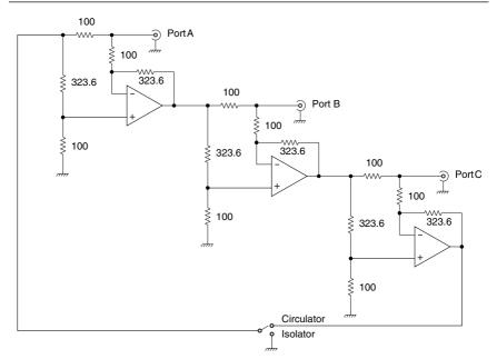
Figure 4.21 The circuit of the active circulator/isolator described in Ref. 1
