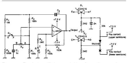
**Figure 2.10** The circuit modified to sound either of two adjacent semitones, according to which key is pressed. The addition of both  $R_6$  and  $R_7$  keeps the loop gain the same when  $S_2$  is closed, leaving the amount of clipping at the rails the same for either semitone (see Figure 2.11(a))
