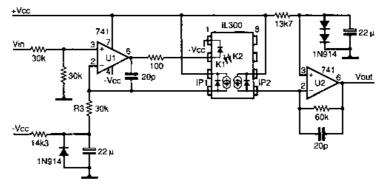
Figure 5.15 Bipolar (prebiased) photoconductive isolation amplifier
