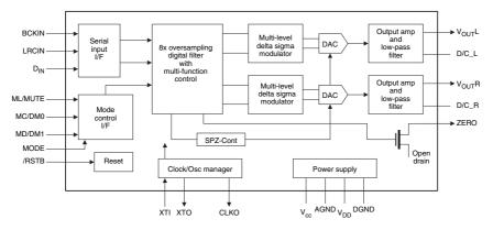
**Figure 1.35** The PCM1717E DAC from Burr-Brown accepts 16 or 18 bit serial data, and provides L and R stereo output channels. With numerous facilities, aimed at CD systems, MPEG audio, MIDI applications, etc.
