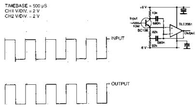
**Figure 3.18** Bootstrapping the emitter circuit as well results in an indistinguishable output
