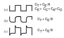
**Figure 3.26** *Displayed waveforms with probe set up (a) correctly, (b) undercompensated, (c) overcompensated*
