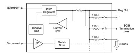
**Figure 1.38** The REG5608 is an 18 line SCSI (small computer systems interface) active terminator chip from Burr-Brown. On-chip resistors and voltage regulator provide the prescribed SCSI bus termination. A single control line open circuits all the terminations, important for 'hot socket' equipment plugging. The device is available in both 28 pin SOIC and fine pitch SSOP packages
