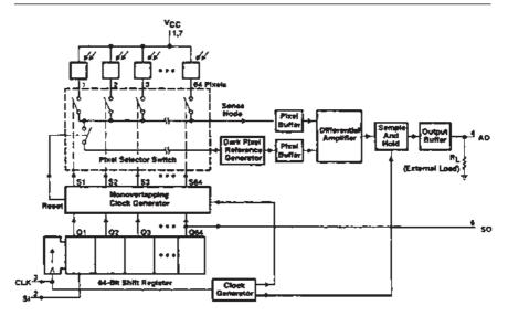
**Figure 5.1** The TSL214 64 element line sensor. The charge stored in each of the 64 pixels during each integration period is read out sequentially via a 64 way mux controlled by the shift register. The charge accumulated in an integration period is proportional to the intensity of the light and the length of the integration period
