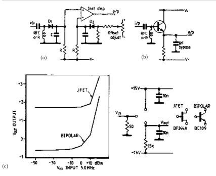
**Figure 4.4** (a) *DC* bias to the diode improves linearity by several dB. If R is made high enough, it becomes a current source greatly extending the linear detection region but this also requires a larger negative rail voltage. (b) Functional equivalent of the diode circuit (a). (c) Comparing the performance of a JFET versus bipolar infinite impedance detector. The latter has a more abrupt cut-off providing a higher dynamic range
