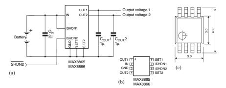
**Figure 1.32** The MAX8865x dual low dropout regulator (a) from MAXIM comes in the proprietary muMAX package, with pinout as at (b). At 3 mm, the package length (c) is similar to TSSOP, but the width across pins is 1.5 mm less, which could lead to its more widespread adoption by other manufacturers
