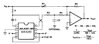
**Figure 3.7** The MAX280/LTC1062 used to create a notch. The input signal can be summed with the filter's output to create the notch
