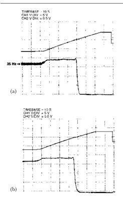
**Figure 3.22** As Figure 3.21(a), but using the MAX294 elliptic filter with its 1.2:1  $F_s$  to  $F_o$  ratio, using a modified detector circuit. (b) As (a), but the detector circuit as in Figure 3.20
