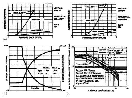
**Figure 6.16** Forward conduction drop of the MCT compared with an IGBT. (b) Modelled and actual turn-off losses of 600 V p-MCT (300 V, +150°C inductive turn-off). (c) Maximum operating frequency as a function of cathode current
