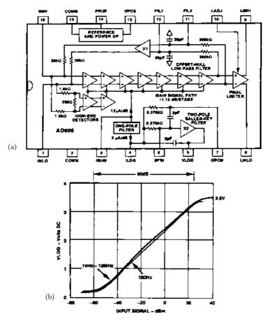
**Figure 1.7** (a) Block diagram of the Analog Devices AD606 50 MHz, 80 dB demodulating logarithmic amplifier with limiter output; (b) shows that the device operates at frequencies down to the audio range
