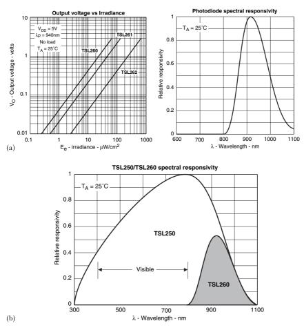
**Figure 5.19** (a) Output voltage as a function of incident illumination for the TSL26x series devices, left, together with spectral response, right. (b) Comparing the spectral response of TSL25x and TSL26x series devices
