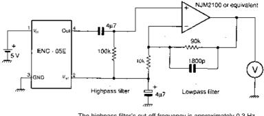
The highpass filter's cut-off frequency is approximately 0.3 Hz The lowpass filter's cut-off frequency is approximately 1 kHz
