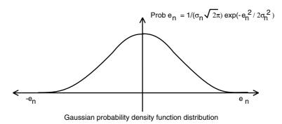
**Figure 7.24** The amplitude distribution of Gaussian white noise, showing how the larger the amplitude, the less likely it is to occur
