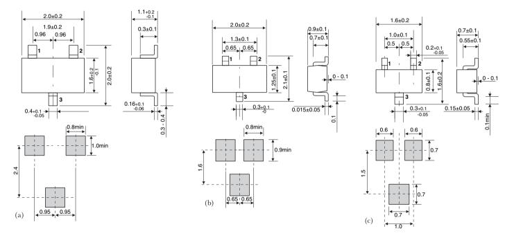
Figure 1.29 Three small transistor outlines: the tiny SOT23-3 (a) dwarfs the SOT323 (b), which in turn dwarfs the minuscule EMT3 (c)
