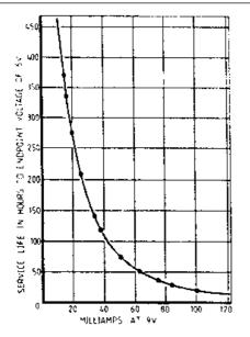
**Figure 6.6** Service life of PP9 battery, used four hours per day
