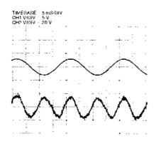
**Figure 5.12** 5 V pp 50 Hz input test signal to the circuit of Figure 5.11 (upper trace) and outphased distortion products (lower trace)
