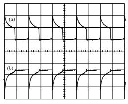
**Figure 5.30** Performance of the circuit of Figure 5.29: (a) collector waveform (upper trace), 2 V/div. vertical, 0 V line at one division above centreline, 10  $\mu$ s/div. horizontal; (b) base waveform (lower trace), 2 V/div. vertical, 0 V line at two divisions below centreline, 10  $\mu$ s/div. horizontal
