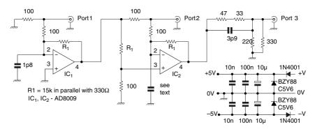
Figure 4.23 Circuit diagram of a wideband isolator, usable from 0 Hz to 500 MHz
