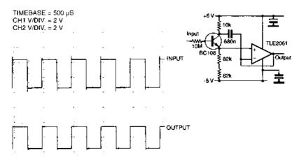
**Figure 3.17** Bootstrapping the emitter follower's collector shortens the input time constant to a negligible value, but the dc gain is still well below unity
