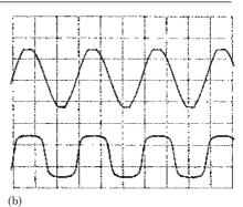
**Figure 2.8** (a) A simple clipper circuit provides an approximation to a squarewave. (b) Comparing the 'squarewave', lower trace, with the input sinewave. (c) Due to the limiting action of the diodes, the ending transient of the squarewave output is extended compared to that of the sinewave
