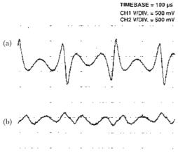
**Figure 2.3** (a) Residual distortion component in OUTPUT 2. Fifth harmonic predominates. (b) Residual after connecting R<sub>11</sub>
