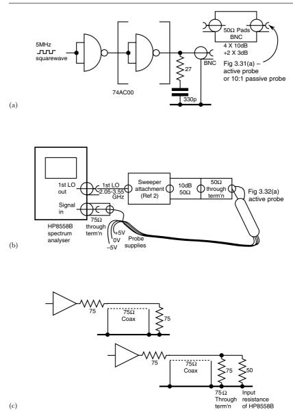
**Figure 3.33** (a) Test circuit used to produce a 5 MHz squarewave with fast edges, to test the probe of Figure 3.31. The 27  $\Omega$  plus 330 pF snubber at the output suppressed ringing on the test waveform. (b) Test set-up used to test the wideband probe of Figure 3.32. (c) Showing how the 6 dB signal reduction in normal use becomes 11 dB in the test set-up of (b) above. Together with the 10 dB pad at the sweeper output, this accounts for the 21 dB separation of the traces in Figure 3.32(b)
