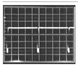
**Figure 5.33** Lightmeter output at a range of 2 cm from the four diodes, on range 5. 1 V/div. vertical, 0 V reference at centreline, 10  $\mu$ s/div. horizontal
