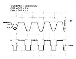
**Figure 5.6** Operating the device in the analog system of Figure 5.5 – 330R load resistor shown in Figure 5.3 removed. Output as a piece of thick card waved back and forth across the sensor (upper trace); output of comparators (lower trace)
