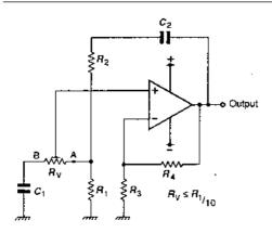
**Figure 2.6** The addition of trimmer potentiometer RV permits tuning of the oscillator without changing the attenuation via the Wien network, provided the resistance of the pot's track does not exceed one-tenth of the reactance of  $C_1$
