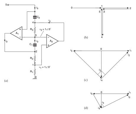
**Figure 1.20** (a) FDNR circuit diagram. If  $v_1$  is the voltage at node 1, etc., then  $v_1 = v_3 = v_5$ . Also,  $i_1 = i_2 = i_3$  and  $i_3 = i_4 + i_5$ . (b) Voltage vector diagram for (a) when  $R_1 = R_2 = R_3 = R$ ,  $C_1 = C_2 = C$  and  $f = \frac{1}{2}\pi CR$ . (c) Current vector diagram for (a), for the same conditions as (b). (d) As (c) but for  $f = \frac{1}{4}\pi CR$ . Note that  $i_2$  and  $i_4$  are always in quadrature.
