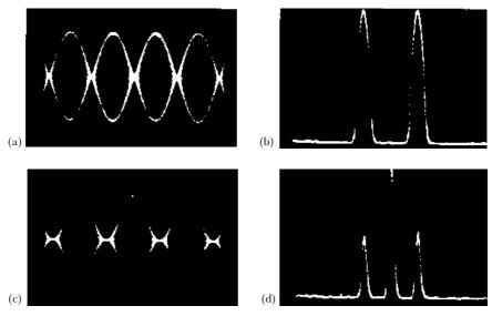
**Figure 7.12** (a) Double sideband suppressed carrier output of the MC1496. (b) Spectrum of (a), rf = 0.5 MHz, baseband modulation 1 kHz. (c) 100% modulation AM, also with rf = 0.5 MHz, baseband modulation 1 kHz. (d) Spectrum of (c)
