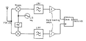
Figure 7.3 Homodyne receiver for frequency-shift keyed transmission
