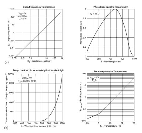
**Figure 5.21** (a) Output frequency versus incident illumination, left, and spectral response, right, for the TSL235 light-to-frequency converter. (b) Temperature coefficient of output frequency of the TSL235, as a function of wavelength, left, and dark frequency performance, right
