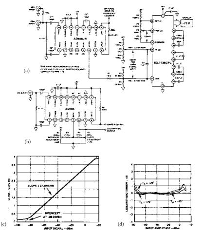
**Figure 1.9** (a) A simple RF power meter using the AD606; (b) AD606 slope and intercept adjustment using pin 5; (c) AD606 nominal transfer function; (d) AD606 log conformance at 10.7 MHz
