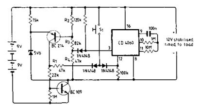
Figure 6.7 Circuit of Figure 6.3, modified to act as stabiliser
