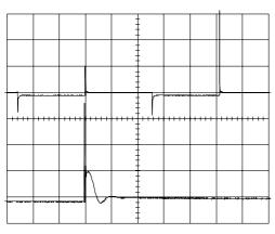
**Figure 6.24** Transient response of the PSU when the load switches between 1 A and 2 A: upper trace 500 mV/div., 200  $\mu$ s/div.; lower trace 500 mV/div., 5  $\mu$ s/div.
