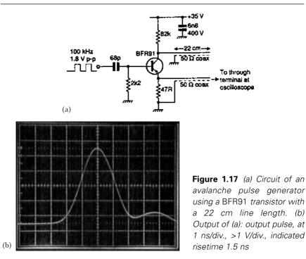
When the quantities must be differenced rms-wise rather than directly, the margin of error is even greater, so no quantitative certainty of the risetime in this case is possible, other than that it is probably well under 1 ns. Unfortunately, a sampling oscilloscope does not feature among my collection of test gear.
