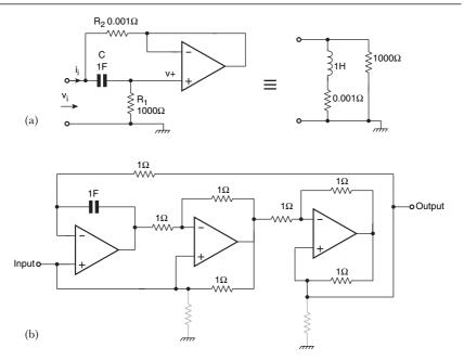
**Figure 1.18** Synthetic inductors. (a) Showing a 1 henry 'inductor' with one end grounded. Q is 10 at 0.00159 Hz, and proportional to frequency above this. Below, it tends to a 0.001  $\Omega$  resistor, just like the corresponding real inductor. (b) Floating synthetic 1 henry inductor. The high value resistors shown dotted are necessary to define the opamp dc conditions if there is no dc path to ground via Input and Output
