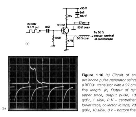
oscilloscope, estimated from the 3 dB bandwidth, is 1.4 ns. Risetimes add rms-wise, so if one were to accept these figures as gospel, it would imply an actual pulse risetime of a little over 500 ps. In fact, the margin for error when an experimental result depends upon the difference of two nearly equal quantities is well known to be large.
