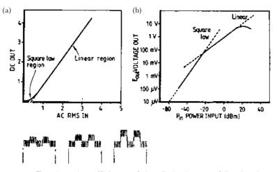
**Figure 4.2** The detection efficiency of the diode detector falls sharply at low signal levels within the square-law region of the diode's response, as the two graphics show. A squarewave modulated carrier can be used to determine sensitivity (see text)
