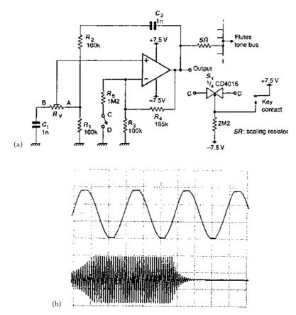
**Figure 2.7** (a) Circuit of a keyed sinewave generator. (b) The output waveform is basically sinusoidal, suitable for use directly for stops of the flute family, upper trace. The starting and ending transients are smooth and free from any incidental dc shift, lower trace
