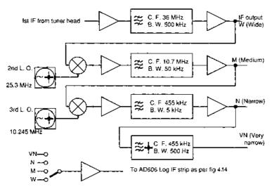
**Figure 4.18** Block diagram showing modified architecture giving a choice of IF bandwidths. It is simpler to provide different signal paths for the different bandwidths rather than select the bandwidth by switching in one or other of several filters all operating at the same IF frequency
