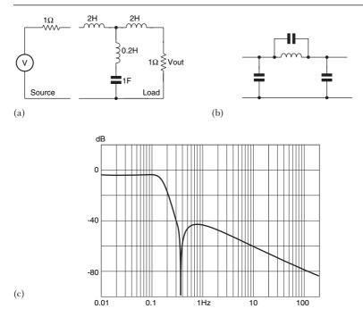
**Figure 1.21** A low component count elliptic lowpass filter with a minimum attenuation of 36 dB from twice the cut-off frequency upwards, the price being as much as 1 dB passband ripple. The minimum capacitor design of (a) is more convenient than (b) for conversion to an FDNR filter. (c) The frequency response of the filter
