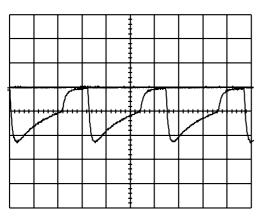
**Figure 5.34** Light output of the circuit of Figure 5.27, measured using range 2 of the lightmeter, at an increased range. 500 mV/div. vertical, 0 V reference line at one division above centreline, 10  $\mu$ s/div. horizontal
