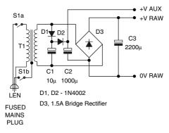
Figure 6.19 The necessary raw and auxiliary supplies
