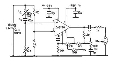
Figure 3.2 Inductance bridge with a 50  $\Omega$  source providing a dc path to ground
