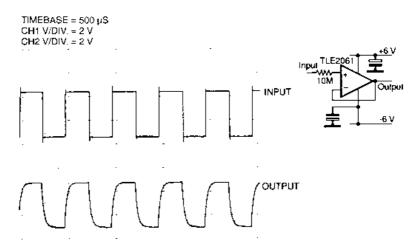
**Figure 3.14** A series 10  $M\Omega$  resistor has no effect on the peak-to-peak amplitude, but grossly limits the high frequency response
