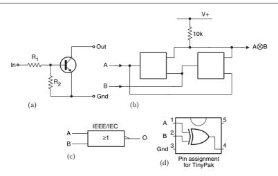
**Figure 1.37** Digital transistors, (a), from Rohm, are available in SOT23 packs (Figure 1.29), with a variety of values for  $R_1$  and  $R_2$ . Two such transistors connected as in (b) give the inverse EXOR or exclusive NOR function. A single component solution is also possible, being readily available in CMOS as the NC7S86M5, (c) and (d), from National Semiconductor
