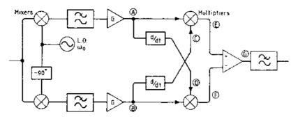
**Figure 7.5** Sine/cosine demodulator, which produces the numerator of equation (7.3) at G
