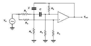
Figure 2.24 The SAB circuit, with finite zero (or notch, above the passband)
