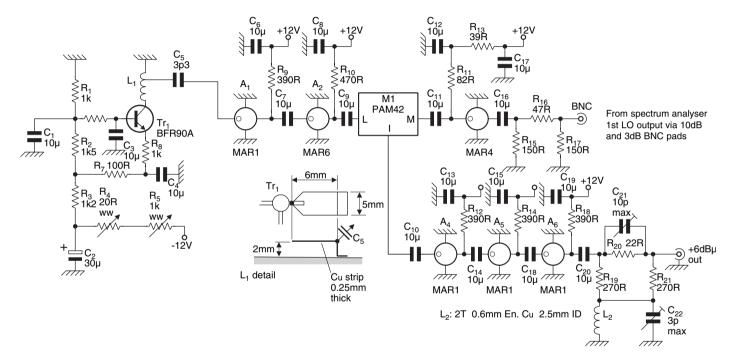
**Figure 4.25** Circuit diagram of an appliqué box for an HP 8558B spectrum analyser, providing a 0–1500 MHz tracking generator output. (Reproduced with permission from Electronic Product Design, July 1994, p.17) (Note: for 10µ read 10n)
