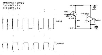
**Figure 3.16** A discrete emitter follower buffer ahead of the opamp improves the high frequency response by a factor of two, but low input resistance pulls down the peak-to-peak output
