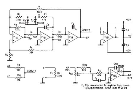
**Figure 2.1** (a) A 1.59 kHz oscillator circuit based on a state variable filter. (A detailed explanation of the SV filter's operation is given in Hickman (1993).) (b) Modifications give a nil net third harmonic at OUTPUT 2
