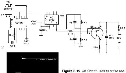
**Figure 6.15** (a) Circuit used to pulse the MCT at 80 A. Note the 100 m $\Omega$  gate drive damping resistor. (b) Gate drive waveform; 10 V/div. vertical, 2  $\mu$ s/div. horizontal (upper trace), voltage across 1  $\Omega$  load, 50 V/div. (lower trace)
