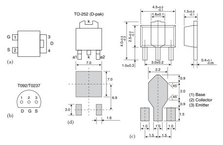
**Figure 1.28** (a) Four pin 0.2' DIP package often used for FETs and other smallpower devices; (b) the TO237 pack is like a TO93, but with a small metal tab extending from the top; (c) the SOT89 pack can typically dissipate 0.5–1 W; (d) the TO252 package dissipates watts – at least at 25°C case temperature!
