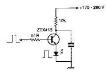
**Figure 1.11** Simple high current avalanche pulse generator circuit, driving a laser diode
