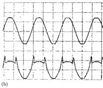
**Figure 2.9** (a) A circuit for adding second (and other) harmonics to the sinewave. (b) The output of the above circuit, lower trace, compared with the sinewave input, upper trace. (c) Showing the fundamental at about 1.7 kHz, the second harmonic about 10 dB down (about right for an open diapason), and many other harmonics. (10 dB/div. vertical, 2 kHz/div. horizontal, span 0–20 kHz)
