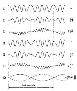
**Figure 7.8** Waveforms seen in the demoduator of Figure 7.5, with a 1 kHz FM signal of peak deviation 7 kHz
