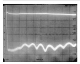
**Figure 4.27** Upper trace as Figure 4.26, for reference. Lower trace, output from port A of the isolator with the input applied to port B. Spectrum analyser settings as for Figure 4.26 except video filter at max.
