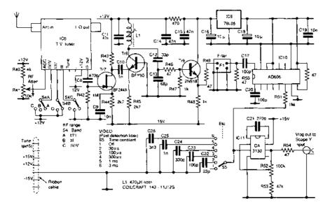
**Figure 4.14** *Circuit diagram of the RF/IF unit. This is built around a Toshiba* EG522F TV tuner, though almost any other model covering Bands I to V inclusive could be used
