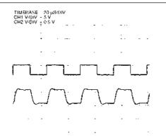
**Figure 5.13** Input and output 1 (Figure 5.11) with a 3.5 V pp 20 kHz squarewave input
