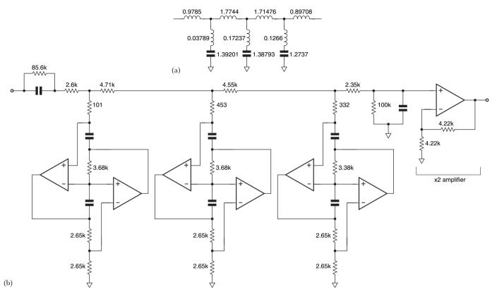
**Figure 1.26** (a) Normalised seven-pole elliptic LC prototype filter, and (b) the derived FDNR input antialiasing filters used in the HP5420A
