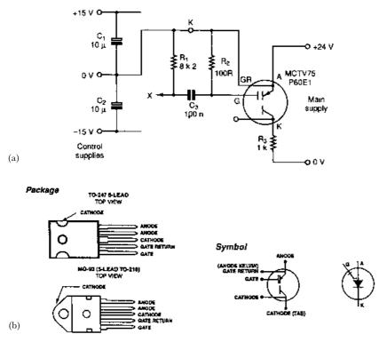
**Figure 6.11** (a) Simple on/off test circuit. (b) Base connections and circuit symbols of the Harris MCT
