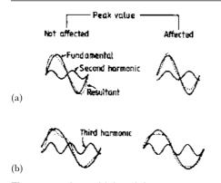
**Figure 4.6** In a wideband detector, measuring the input signal's positive peak may affect the expected ratio of peak-to-rms voltage. (a), (b) show resultant phases in second and third harmonics
