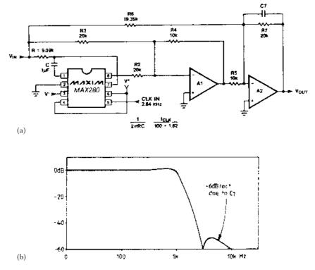
**Figure 3.9** Modifying the lospass filter circuit, (a) with  $R = 39 k\Omega$ , C = 5n6,  $C_7 = 1 n$ ,  $R_{2,3,6,7} = 100 k\Omega$  and  $R_{4,5} = 47 k\Omega$  gives the response shown in (b)
