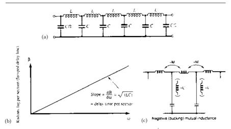
**Figure 1.2** (a) Basic delay line – (b) providing a delay of  $\sqrt{(LC)}$  seconds per section at dc and low frequencies. (c) Connection of negative inductance in the shunt arms to linearise the group delay over a larger proportion of the filter's passband. Not a physical component, it is implemented by negative mutual inductance (bucking coupling) between sections of series inductance
