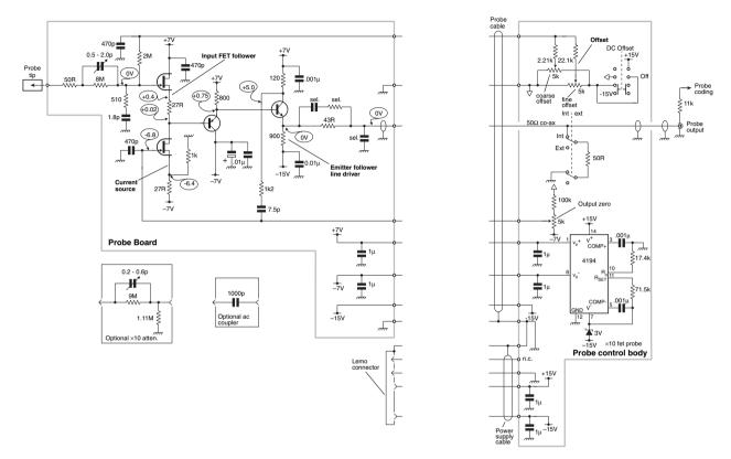
**Figure 3.28** Circuit diagram of the P6202A active FET input probe, with a dc – 500 MHz bandwidth and 2 pF input capacitance (Courtesy Tektronix UK Ltd)
