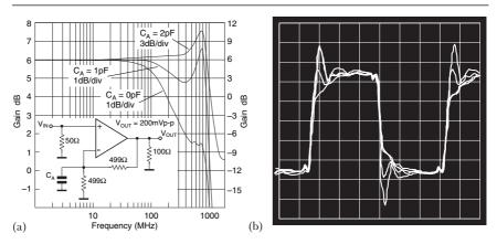
**Figure 4.24** (a) Bandwidth extension for the AD8009 achieved (for a gain of +2) by adding capacitance from the inverting input to ground. (b) The effect of these three values of capacitance on the pulse response
