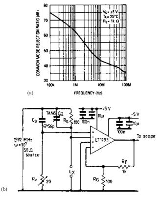
**Figure 3.4** (a) Common mode rejection ratio versus frequency for the LT1193. (b) The 'hastily constructed' circuit using the LT1193 in a bridge application
