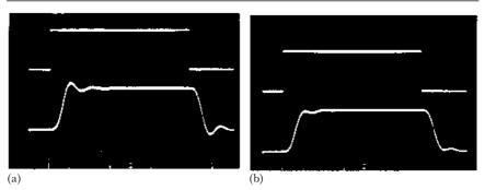
**Figure 3.8** Using a lowpass filter to give an approximation to (a) a Butterworth and (b) a Bessel step response
