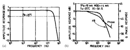
**Figure 5.14** Bandwidth of the IL300 optocoupler: (a) in photovoltaic mode; (b) in photoconductive mode
