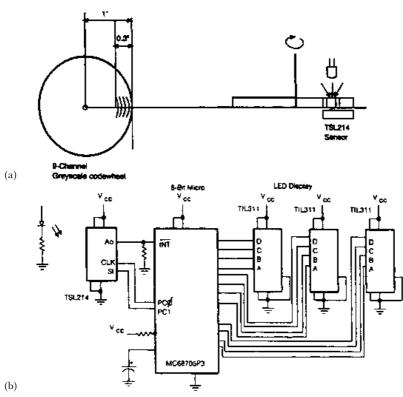
**Figure 5.8** Mated with a 9 channel grey-scale codewheel, the TSL214 can provide rotary position readout to better than 1° resolution (a), or display shaft position in degrees (b)
