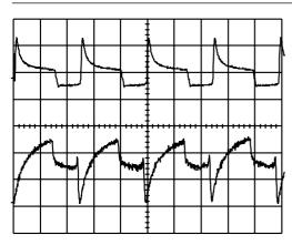
**Figure 5.26** Variation of light output from an uncoated fluorescent lamp. Photodiode at 30 cm from the tube, lightmeter set to range 3. Lower trace: light output as measured by circuit of Figure 5.23, 5 ms/div. horizontal, 0.2 V/div. vertical, 0 V at centreline. Upper trace: waveform of the voltage applied across the tube, via capacitive pick-up, 5 ms/div. horizontal, 2 V/div. vertical, 0 V at two divisions above centreline
