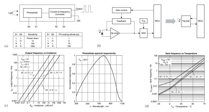
**Figure 5.22** (a) Functional block diagram of the TSL230 programmable light-to-frequency converter. (b) Illustrating the system simplification possible with the TSL230 programmable light-to-frequency converter. (c) Illustrating the various sensitivity ranges available to the user with the TSL230, left, together with spectral responsivity, right. (d) Showing the very low dark frequency output of the TSL230, as a function of temperature
