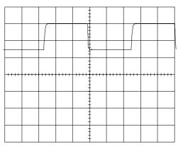
**Figure 6.23** Load switching between 33  $\Omega$  and 17.5  $\Omega$ , with the demanded output voltage set to 15 V but the current limit reduced to roughly 0.5 A, i.e. such that at 17.5  $\Omega$  the voltage collapses to 7.5 V: 5 V/div., centreline = 0 V, 200 µs/div.
