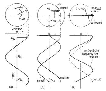
**Figure 7.2** Vector representation of sinusoidal waveforms. Waveform at (a) is derived from projection of rotating vector onto horizontal axis, while at (b) two such vectors are shown in quadrature, producing sine and cosine waves. Slightly different frequencies produce the effect seen at (c)
