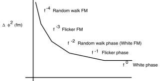
Fourier frequency (sideband-, offset- or modulation-frequency)
