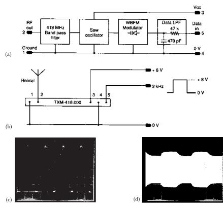
**Figure 7.15** (a) Block diagram of the TX-UHF transmitter module. (b) Connections in recommended test circuit. (c) The output of the transmitter module following 20 dB of attenuation, 10 mV/div. vertical, 1 ns/div. horizontal, 12 V supply, no modulation. (d) As (c) except 9 V supply, 100  $\mu$ s/div. horizontal, 2.4 kHz squarewave modulation applied
