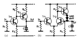
**Figure 4.5** (a), (b) Active detectors provide further improvements on the infinite impedance detectors
