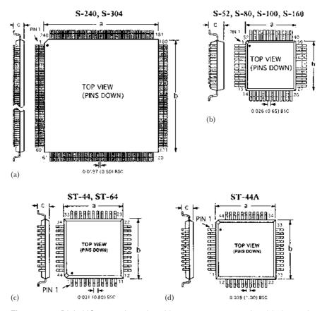
**Figure 1.36** Digital ICs come in packs with up to 300 or more pins. (a) shows the 240 pin PQFP (plastic quad flat package) S-240. The slightly wider pin spacing of PQFP packs with up to 160 pins, (b), is more manageable. There are traps for the unwary! The two 44 pin TQFP (thin quad flat package) packs in (c) and (d) look very similar, but the pin spacing is different
