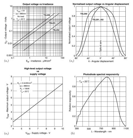
**Figure 5.18** (a) Output voltage as a function of incident illumination for the TSL25x series devices, top, with curves for maximum output against supply, bottom left, and spectral responsivity, right. (b) Angular response of the TSL25x series devices
