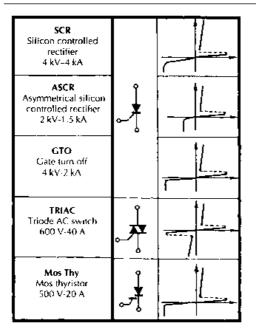
**Figure 6.9** Variations on the silicon controlled rectifier theme. (Reproduced by courtesy of Motorola Inc.)
