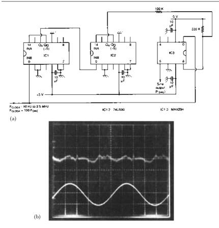
**Figure 3.23** (a) Circuit of a digitally tuned sinewave audio oscillator using the MAX294. (b) The circuit's output at 1 kHz (lower trace) and the residual signal after filtering out the fundamental, representing the total harmonic distortion (upper trace)
