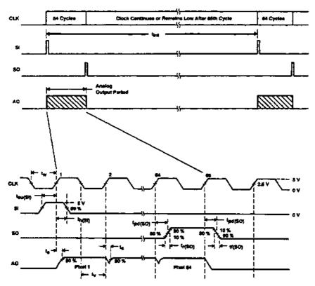
**Figure 5.2** The pixel outputs appear sequentially on the A<sub>o</sub> pin following the rising edges of the next 64 clock pulses that follow the assertion of the SI pulse, assuming its set-up and hold times are met. Following the sample time  $t_s$ , the pixel analog data is valid for at least the period  $t_v$
