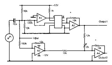
**Figure 5.11** Test circuit used for evaluating the IL300 operating in positive unipolar photovoltaic mode. Ideally, there should be zero resultant signal at output 2
