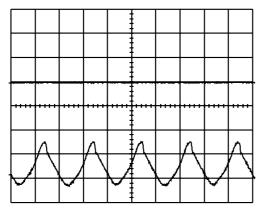
**Figure 5.25** Variation of light output from a 'white' fluorescent lamp. Photodiode at 50 cm from the tube, lightmeter set to range 3. Oscilloscope settings 5 ms/div. horizontal, 0.2 V/div. vertical
