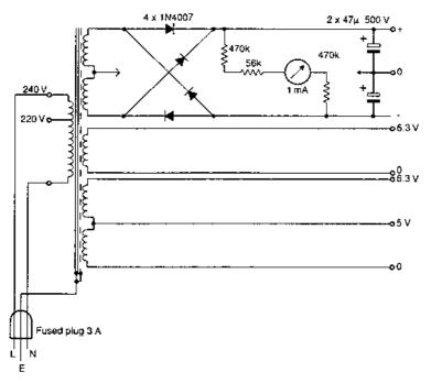
**Figure 1.12** High-voltage power supply, using a mains transformer from the days of valves
