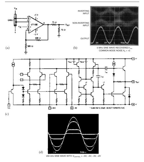
**Figure 3.3** (a) Cable sense amplifier for loop through connections with dc adjust. (b) Recovered signal from common mode noise. (c) LT1193 simplified schematic. (d) Sinewave reduced by limiting the LT1194
