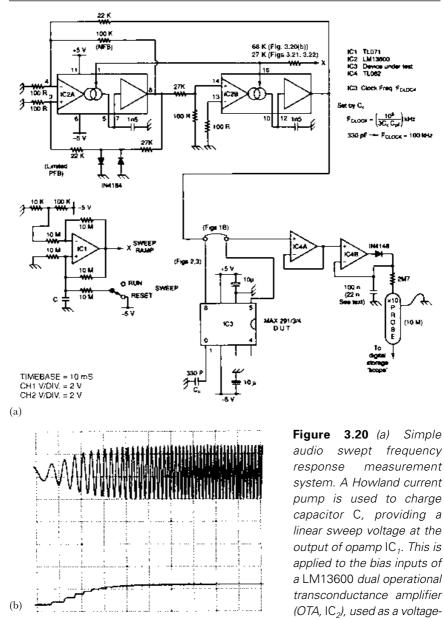
controlled state-variable-filter based sinewave oscillator. Its output is applied to the device under test,  $IC_3$ , the output of the latter being detected by the ideal rectifier circuit  $IC_4$ . (b) Using a small value of C, the swept oscillator output was applied direct to the detector circuit. The detected output (lower trace) follows faithfully the peak amplitude of the sweeper output (upper trace) over the partial scan shown, covering about 30 Hz to 650 Hz
