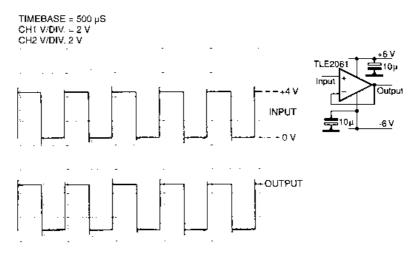
**Figure 3.13** JFET input unity gain buffer circuit's output is indistinguishable from its input
