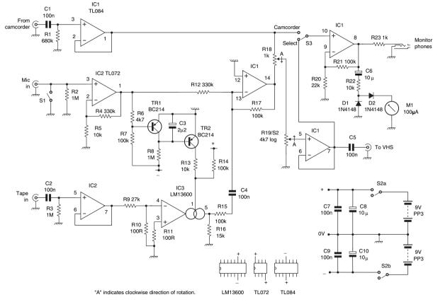
**Figure 2.27** The circuit diagram of the appliqué box, for HI8 to VHS sound dubbing
