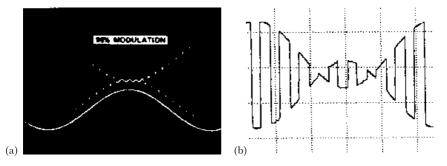
**Figure 7.13** (a) AM with modulation index of 96%. The waveform is continuous with no sudden phase changes. (b) AM with modulation index of 130%; instantaneous 180° phase flips are visible twice per cycle
