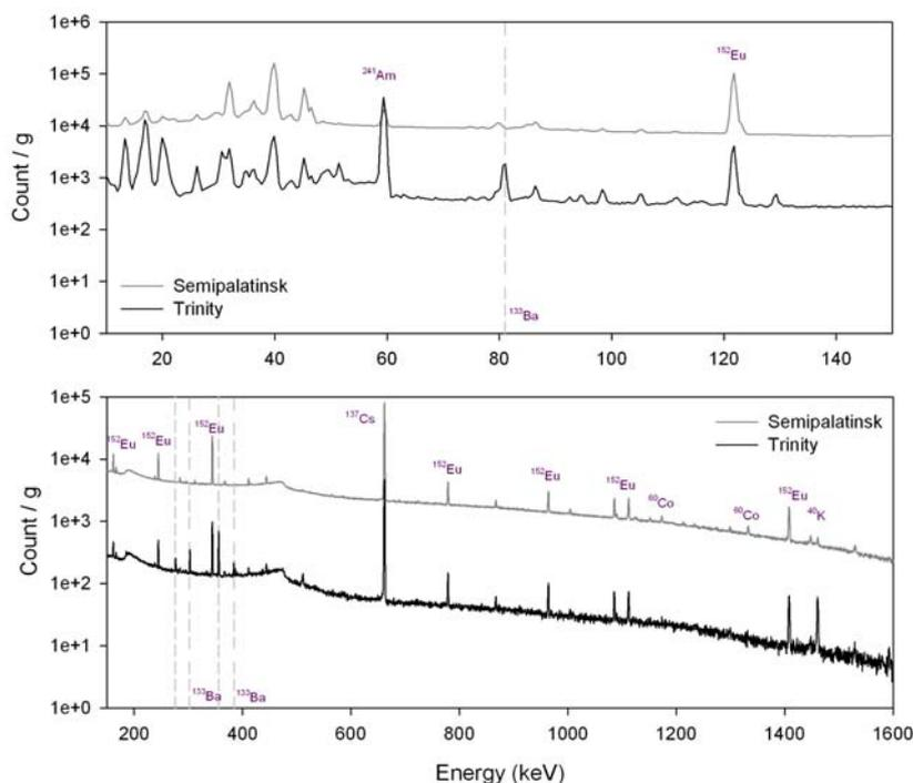
Fig. 5. 24 hour comparison spectra of atomsite from Semipalatinsk and Trinitite (sample #26) measured by Ortec LO-AX HPGe detector. Dashed lines indicate the main  $^{133}\text{Ba}$  gamma lines in Trinitite and the lack of  $^{133}\text{Ba}$  in the sample from Semipalatinsk.
