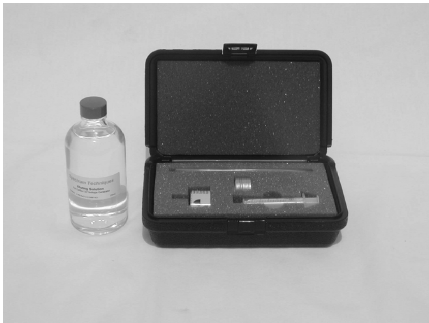
Figure 3: Isotope Generator to make Ba-137m from Cs-137
