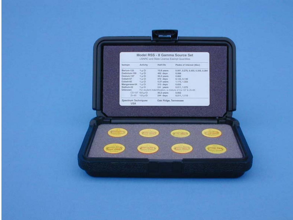
Figure 3: Kit of eight different gamma sources.
