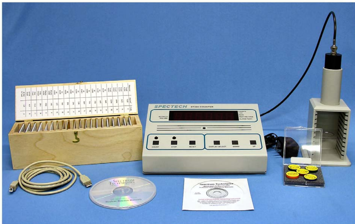
Figure 2: ST360 setup with sources and absorber kit.
