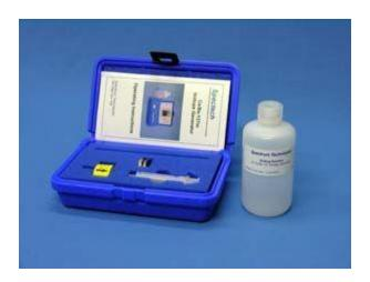
The parent isotope Cs-137 with a half-life of 30.1 years beta decays (94.6%) to the metastable state of Ba-137m. This further decays by gamma emission (662 keV) with a half-life of 2.6 min. to the stable Ba-137 element. During elution using a solution of 0.9% NaCl,, the Ba-137m is selectively "milked" from the generator leaving behind the Cs-137 parent. Regeneration of the Ba-137m occurs as the Cs-137 continues to decay, reestablishing equilibrium in less than 1 hour.
